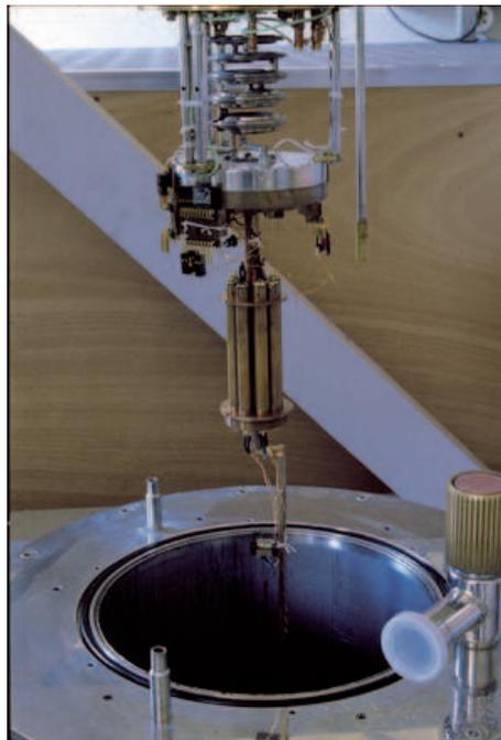
Figure 85: Lower part of the cooling finger of a dilution refrigerator.
