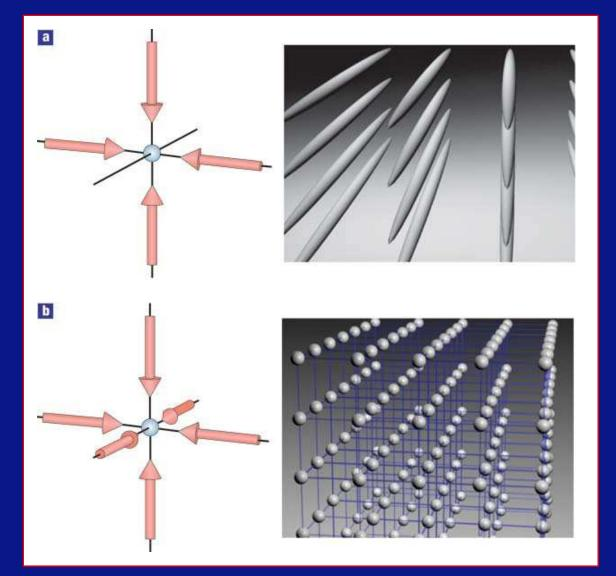
Counterpropagating lasers:  $\longrightarrow$  standing light field. **Trap potential** varies as  $U_{\rm lat} \sin^2(\vec{k}\vec{r})$ with  $k = \frac{2\pi}{\lambda}$  $\lambda$ : laser wavelength.  $U_{\rm lat} \propto I \, \alpha(\lambda)$ with laser intensity I and atomic polarizability  $\alpha$ .
