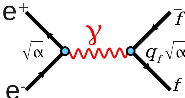
$$f\bar{f}: e^+e^-, \mu^+\mu^-, \tau^+\tau^- \quad c_f = 1 \quad \sigma_f = c_f q_f^2 \sigma_0 \quad \sigma_0 = \frac{4\pi\alpha^2}{3s}$$
