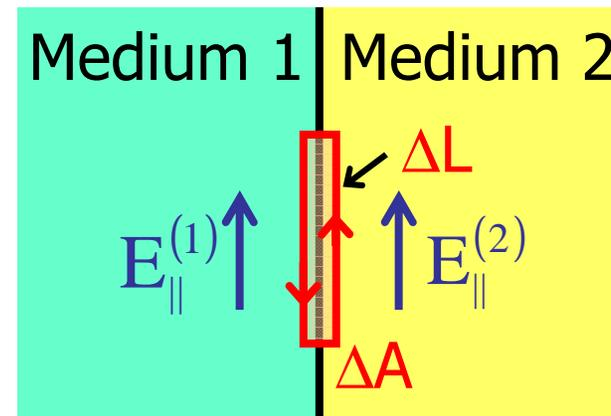
$$\begin{aligned} 0 &= \int \text{rot } \vec{E} d\vec{A} = \oint \vec{E} d\vec{s} \\ &= (\vec{E}_{\parallel}^{(2)} - \vec{E}_{\parallel}^{(1)}) \cdot \Delta \vec{L} \end{aligned}$$
