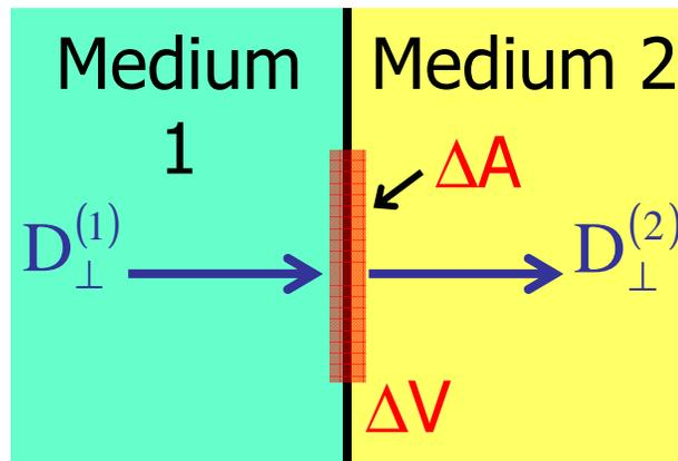
$$\begin{aligned} 0 &= \int \text{div } \vec{D} dV = \oint \vec{D} d\vec{A} \\ &= (\vec{D}_{\perp}^{(2)} - \vec{D}_{\perp}^{(1)}) \cdot \Delta \vec{A} \end{aligned}$$
