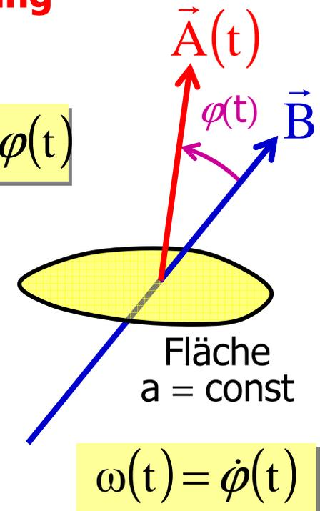
$$\omega = \text{const.}, \quad \varphi(t) = \omega t \Rightarrow U_{\text{ind}} = B A \omega \sin(\omega t)$$
