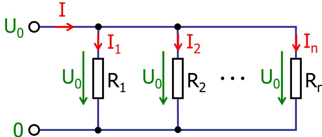
Knotenregel:  $-I + I_1 + I_2 + \dots + I_n = 0 \Rightarrow \frac{U_0}{R_{\text{tot}}} = \sum_{i=1}^n \frac{U_0}{R_i}$
