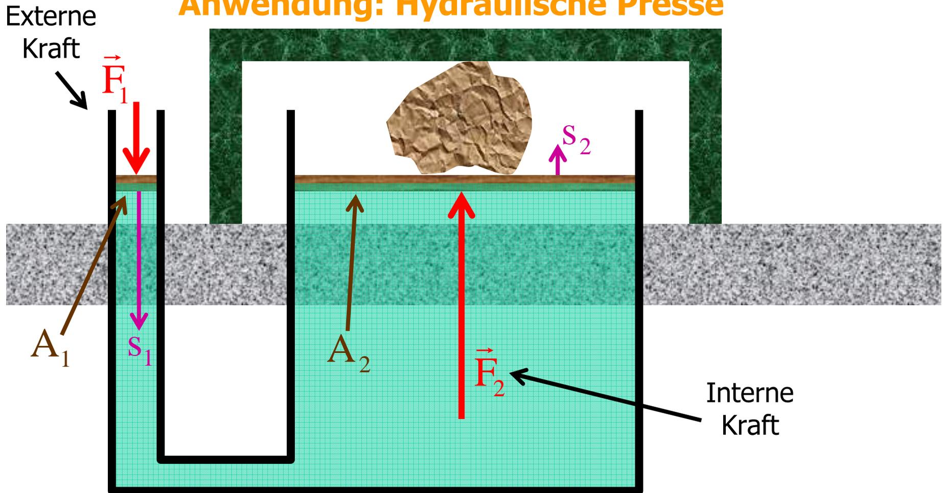
$$p = \frac{F_1}{A_1} = \frac{F_2}{A_2} \Rightarrow F_2 = \frac{A_2}{A_1} F_1 \gg F_1 \quad \text{aber} \quad s_2 = \frac{A_1}{A_2} s_1 \ll s_1$$
