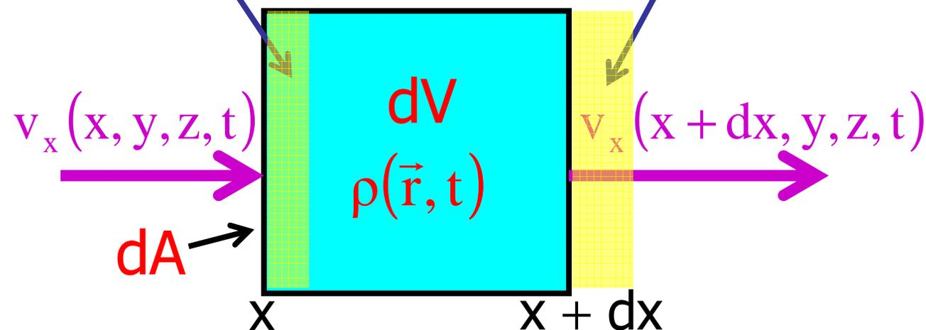
$$dm \Big|_x = dm \Big|_{\text{in}} - dm \Big|_{\text{aus}} = - \frac{\partial}{\partial x} (\rho v_x) \cdot \underbrace{dx \cdot dA}_{dV} \cdot dt$$
