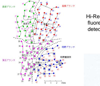
AGASA (Akeno, Japan) 100 km<sup>2</sup> ground array Sketch of ground array with fluorescence detector – Auger Project realizes this concept
