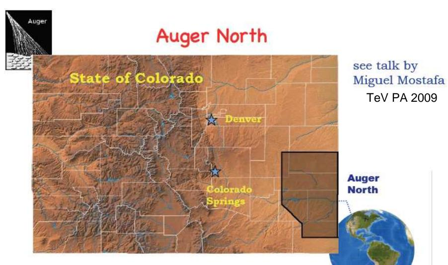
Auger North: 4400 detectors 1.42 mi Square Grid 21,000 km<sup>2</sup> (8000 mi<sup>2</sup>) Auger South: 1600 detectors 1.5 km Triangular Grid 3000 km<sup>2</sup> (1200 mi<sup>2</sup>)
