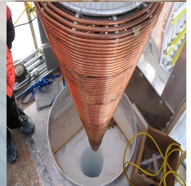
**Drill with hot water under high pressure
