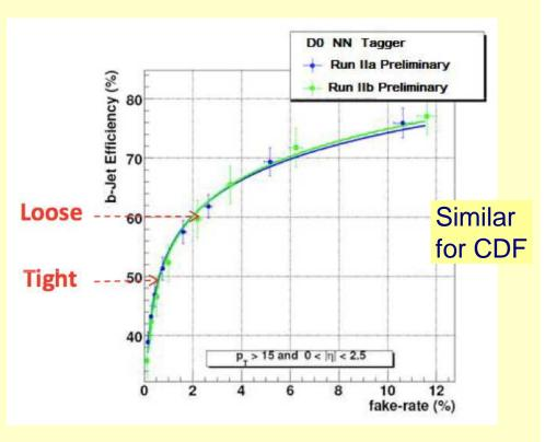
Neural networks are used for optimal combination of tagging information
