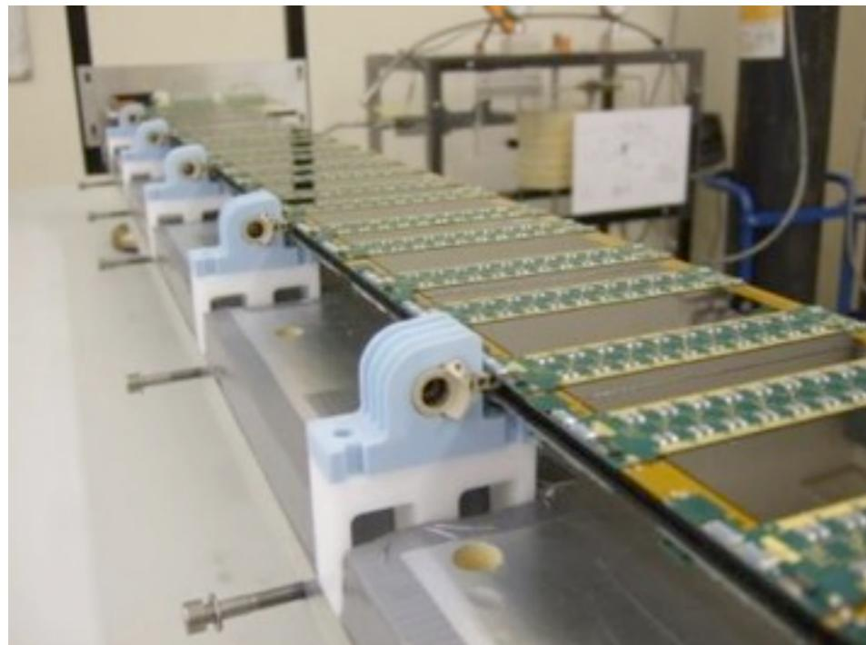
Full-size demonstrator made with realistic mechanical modules, stave cores, bus cables and locking mechanism. It is cooled to -35 C° with a CO<sub>2</sub> blow system. During cooling from room temperature to operating temperature, deflections less than 100  $\mu\text{m}$  were measured.
