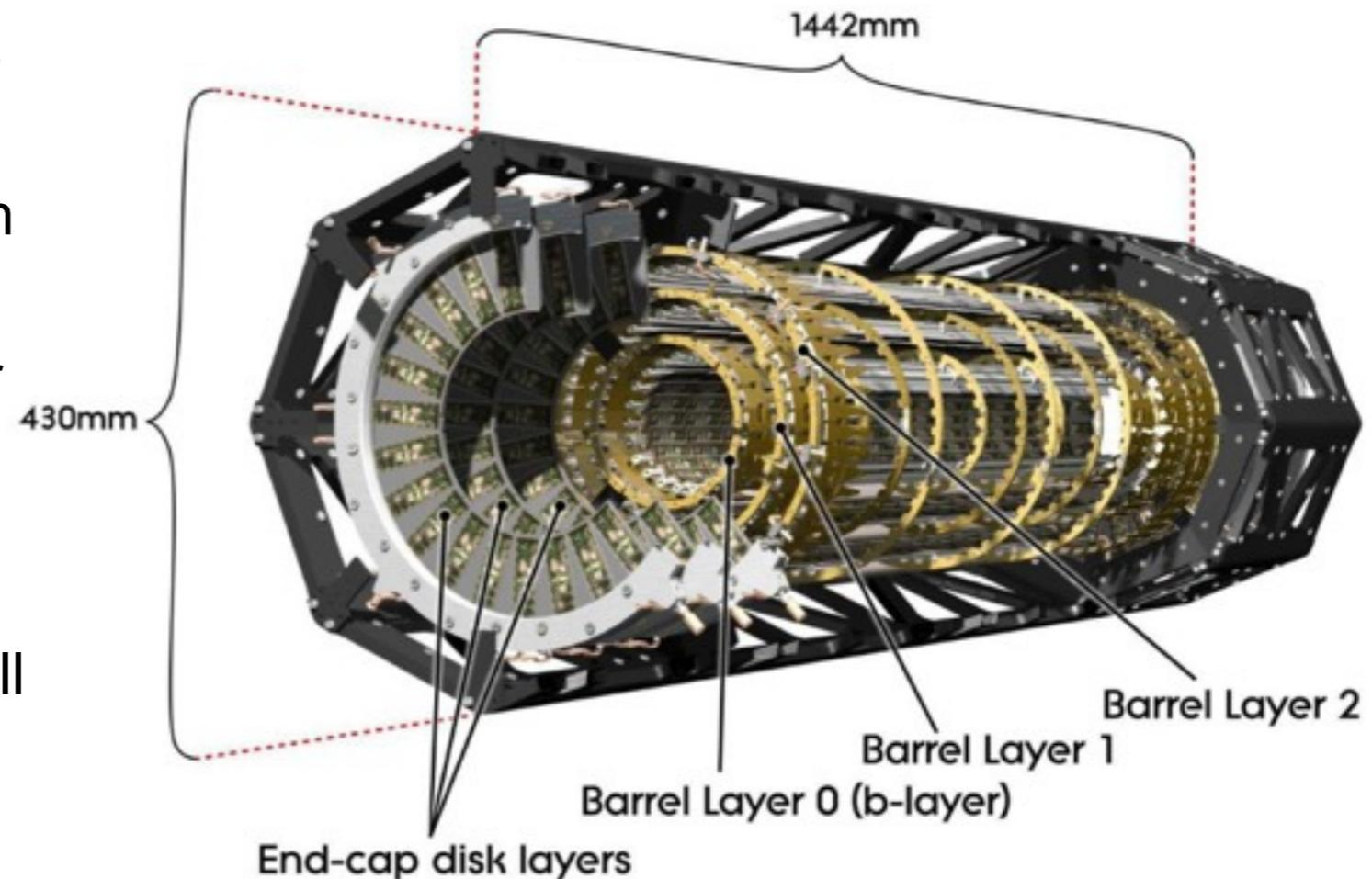
The same module is used in the barrel and in the disks:
