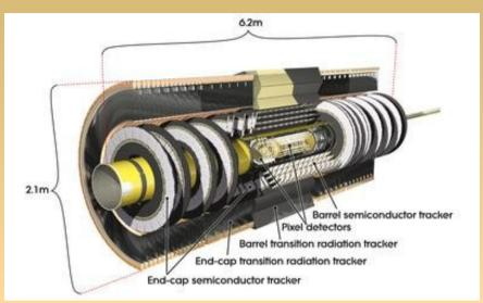
Si strips modules each with 4 detectors (2 on each side), 6.3 million readout channels
