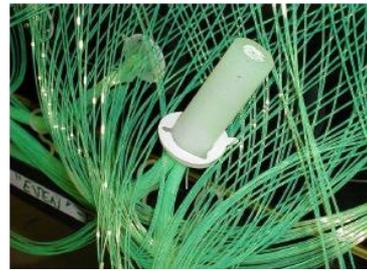
optical signals read out with PMTs
