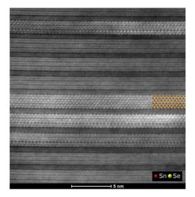
**Above**. Representative cross-section STEM-HAADF image of a[(SnSe)1.15]3(VSe2)1 sample. The image clearly contains a brighter set of three bilayers corresponding to the SnSe layers and a darker VSe2 layer. A structural model of SnSe along [010] is inset on the right of the image.
