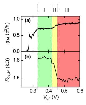
**Above**. Transport in a QR with QPCs embedded in the leads: (a) Two-terminal conductance g14 as a function of  $V_{g1}$  at T = 23 mK and  $V_{g2}$  = 650 mV. (b) Four-terminal, non-local resistance R21,34 as a function of Vg1 at T = 23 mK and Vg2 = 650 mV. The regions I and III indicate transport in the first and second subbands of QPC1, respectively. Region II indicates the transition between the two subbands.
