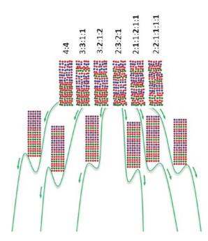
**Above**. Schematic representation of the free-energy landscape for the formation of the six isomers of  $[(PbSe)_{1,14}]_4(NbSe_2)_4$ . The images at the top depict the structures of the initial reactants. The images in the middle depict idealised atomic structures of the six isomers formed on annealing. The green lines show the energy pathways for the six different reactants transforming into the six different targeted compounds.
