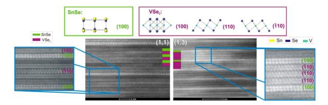
**Above**. HAADF-STEM images of the samples ( $[SnSe]_{1.15}$ )<sub>1</sub>( $VSe_2$ )<sub>n</sub> with n = 1 and 3. The different crystallographic orientations of the individual layers are highlighted.
