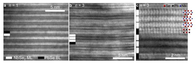
**Above**. Cross-sectional HAADF-STEM images of  $(PbSe)_{1.14}(NbSe_2)_n$  ferecrystals. (a) The layer structure is shown on the atomic scale for n = 1. A NbSe<sub>2</sub> monolayer (ML) is indicated by a white bar and a PbSe atomic bilayer (BL) is indicated by a black bar. (b) HAADF-STEM image of n = 3. (c) High-resolution HAADF-STEM image of n = 3 showing single atomic columns. The atomic columns resolved in the PbSe layer agree with a projection of bulk PbSe along the [100] direction.
