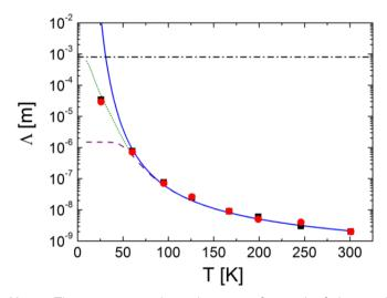
**Above**. The temperature dependent mean free path of phonons in the insulating Magnesium-doped  $\beta$ -Ga<sub>2</sub>O<sub>3</sub>. The solid line is the theoretical contribution for phonon-phonon-Umklapp-scattering and the dashed line shows additionally a contribution of a second scattering process with a constant mean free path of 1:5  $\mu$ m. The dotted line describes point-defect-scattering within the scope of Rayleigh scattering.
