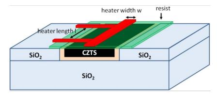
**Above**. Schematic measurement setup containing the kesterite CZTS crystal glued and polished between two glass wafers. An electrically insulating photoresist of about  $1 \,\mu$ m is placed on top of the crystal. A photolithographic designed gold heater line is placed on top of the resist.
