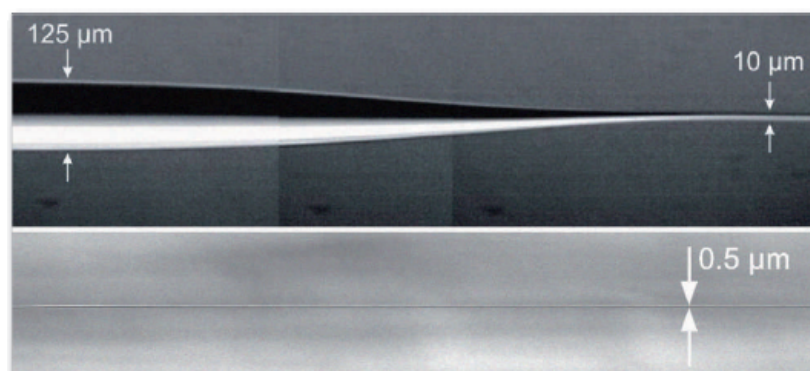
Fig. 1.2 (top) Scanning electron microscope (SEM) picture of the taper transition from a standard fiber diameter to the nanofiber part. For a waist of 10 mm length the taper region is about 35 mm on each side to guarantee an adiabatic transition of the electromagnetic field mode. (bottom) Waist of the nanofiber, true to scale. Taken from (Rauschenbeutel (2009))
