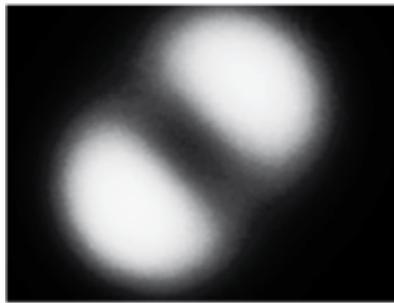
FIGURE 4.6: The superposition of higher order modes in a fibre creates a butterfly-shaped mode.
