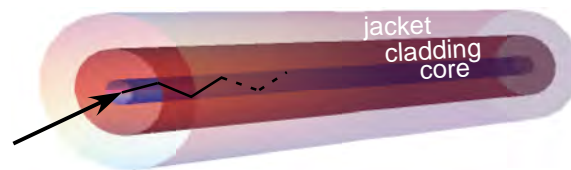
Figure 2.1: Standard optical fiber. Nomenclature for describing a standard optical fiber. A light ray (black line) is totally internally reflected inside the core (blue) due to its higher refractive index with respect to the cladding (red). To protect the waveguide from its surrounding environment it is usually coated with a jacket layer.
