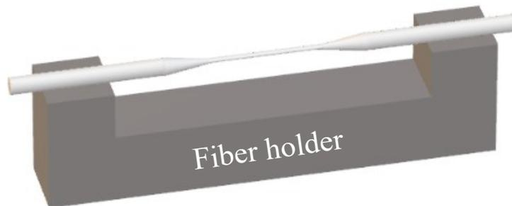
Figure 16: Schematic of the customized nanofiber holder where the two tapered ends are attached with UV curing glue.
