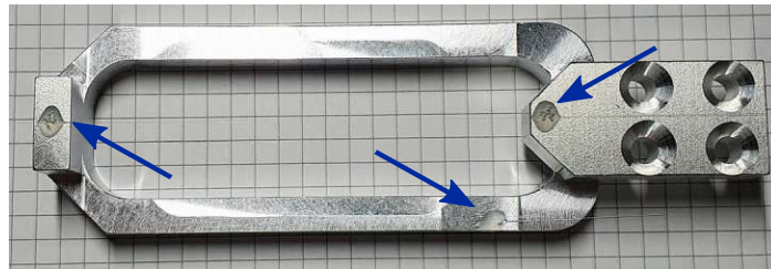
Fig. 3.7 Picture of the fibermount used for the first fiber, after it has been replaced in Berlin. One can clearly see the two glue points placed centrally to fix the fiber and one on the side of the frame to safely guide the fiber to the back of the chamber.
