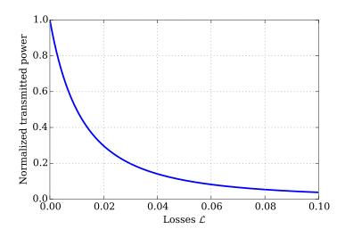
Figure 2.22: Change of transmitted power on resonance ( $\Delta \phi = 0$ ) when increasing the losses within the resonator. These losses comprise losses due to the medium as well as losses during reflection or transmission at the mirrors. Basis for this graph is equation 2.74 with  $T_1 \approx T_2 \approx 0.012$ , as for the cavity used in this report.
