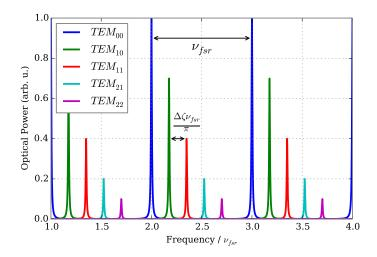
Figure 2.12: Example of coupling to the fundamental mode (TEM<sub>00</sub>) as well as higher-order modes. The frequency spacing between the fundamental modes is the FSR and between higher-order modes with (l + m - l' - m') = j is  $j \frac{\Delta \zeta \nu_{\text{fsr}}}{\pi}$ . The relative frequency spacings are chosen to match the ones of the cavity used in this report and the relative strength of the transverse modes is arbitrarily scaled.
