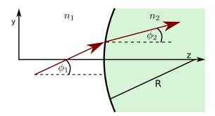
Figure 2.8: Rays propagating in positive z direction can be fully characterized by their angle  $\phi$  with the optical axis (z axis) and their distance y from the z axis. Any optical component might change the ray's coordinates  $(y, \phi)$ .
