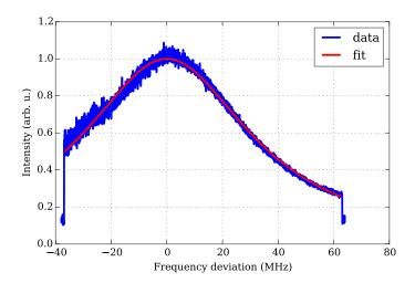
Figure 2.16: Transmission through cavity in dependence of detuning from resonance frequency. Shown are the data (blue) and a Lorentzian fit (red). The data is obtained with a single-photon counting module and already corrected for the change of diffraction efficiency of the AOM.
