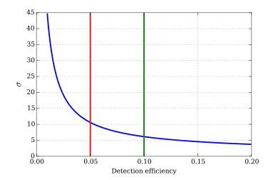
Figure 3.15: Influence of detection efficiency on variance estimation. The variance is calculated with equation 3.29 for 30 trapped atoms. The vertical lines correspond to the current detection efficiency (red) and the achievable detection efficiency (green) when bypassing the 50:50 beamsplitter in front of the cavity (see figure 3.1). Detection efficiency means the probability of detecting a photon that is in the nanofiber and propagates towards the detector.
