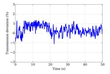
Figure 2.32: Short-term stability of the intensity after the cavity. Shown is the deviation from the mean of all data in percent. Note that this is not a zoom of the data shown in 2.29 but is a different measurement.
