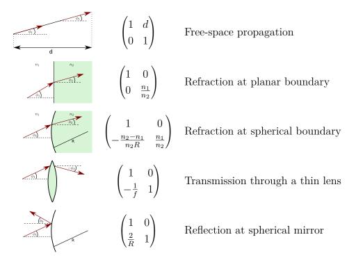
Table 2.1: Some important ray transfer matrices that will be used in later sections. Note that the focal length f is positive and the radii R are defined as positive if the ray impacts on a convex boundary and negative for concave boundaries.
