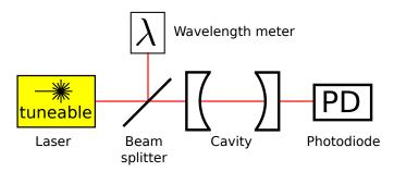
Figure 2.13: Sketch of the setup to measure the FSR. The tuneable laser is coupled into the cavity and the transmission measured with a photodiode. At the same time, the frequency of the laser is measured with a wavelength meter. Note that this setup is just a sketch and is missing the coupling mirrors as well as the coupling lens (cf. section 2.3.8).
