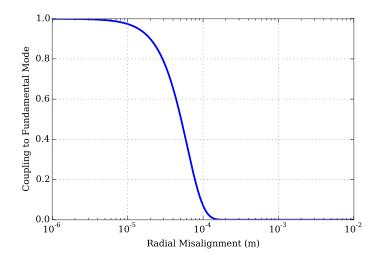
Figure 2.18: Change of coupling efficiency to fundamental mode with radial misalignment of the beam. The misalignment is assumed to be in such a way that the beam is always parallel to the optical axis. This calculation is based on a focal lens of 175 mm placed 174 mm before the center of the cavity.
