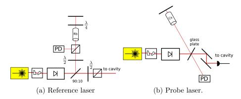
Figure 2.28: Laser setup with saturation spectroscopy.
