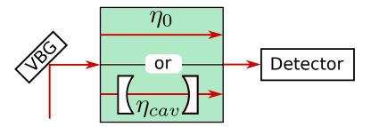
Figure 2.21: Schematic setup for measurement of background suppression. The beam is filtered by a volume Bragg grating before either being directly routed to the detector or filtered by the cavity before detection.  $\eta_0$  and  $\eta_{\text{cav}}$  are the factors introduced in equations 2.66 and 2.67.
