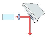
Figure 2.27: Littrow configuration for an ECDL. The angle and position of the Bragg grating (dark gray) can be adjusted with a micrometer screw and a piezo-electric actuator (not shown).
