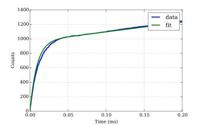
Figure 3.3: Fitting equation 3.23 to the total detector counts with free parameter  $N_{\rm A,0}$ . The actual number of initially trapped atoms for this simulation was 1000 and the fit yielded 1088.
