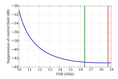
Figure 2.15: Suppression of the control field in EIT when transmission is maximized for the probe field. The calculation is based on equation 2.36 and the frequency spacing between control field and probe field is 9.2 GHz (cf. section 2.1.2). A finesse of 223 is assumed (cf. section 2.3.7). The two vertical lines mark the actual FSR of 16.42 GHz (green) and the ideal FSR of 18.7 GHz (red).
