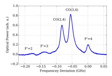
Figure 2.26: Saturation spectroscopy of Rubidium 85. Shown are the hyperfine transitions  $F=3\to F'$ . This corresponds to to the transitions shown in figure 2.25 when correcting for the Doppler-broadened background. CO(3,4) means the crossover peak of transitions  $F=3\to F'=3$  and  $F=3\to F'=4$ . The x-axis shows the frequency deviation from the Rubidium 85 D2  $F=3\to F'=4$  transition.
