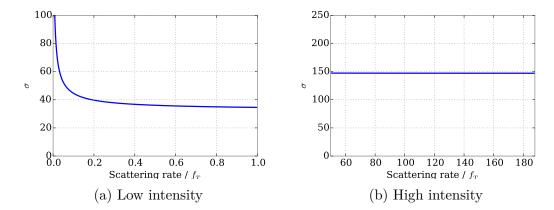
Figure 3.13: Square-root of variance as calculated with equation 3.29 in dependence of the scattering rate for 1000 atoms.  $f_T$  is the lowest trap frequency (87 kHz). The calculations are done using the optimal pulse time for each scattering rate as described in section 3.3.3. The maximal scattering rate of  $\frac{188}{f_T}$  in (b) corresponds to  $\frac{\gamma}{2}$ , where  $\gamma$  is the natural linewidth.
