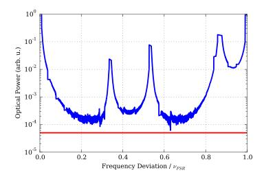
Figure 2.19: Measured optical power behind the cavity while scanning over one FSR. The x-axis shows the deviation from the fundamental mode. 3 transverse modes can be seen. This measurement is taken directly after the cavity. Note that the resolution is not very high and thus some "edgy" parts can be seen. Note also that this is early data and the coupling to the fundamental mode has since been improved (see text).
