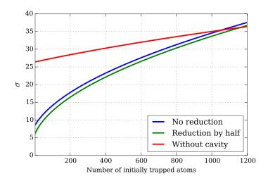
Figure 3.14: Standard deviation (cf. equation 3.29) in dependence of atom number. The graphs show the effects of a reduction of background counts by a factor of 2 and the effect of the cavity.
