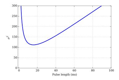
Figure 3.6: Variance of the number of initially trapped atoms in dependence of measurement time. The minimal variance of 112 is at  $t = 16 \,\text{ms}$ . This calculation is for 30 atoms.
