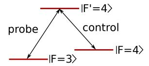
Figure 2.6: Lambda level scheme for EIT. A probe beam drives the  $|F=3\rangle$ - $|F'=4\rangle$  transition and a control field the  $|F=4\rangle$ - $|F'=4\rangle$  transition. In this case, cesium atoms were used and the levels correspond to the hyperfine states of the D2 line.
