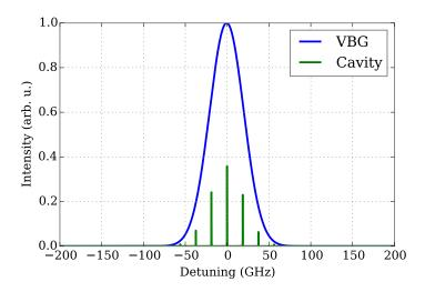
Figure 2.4: The light from the volume Bragg grating (VBG) shows a Gaussian distribution on a frequency axis (blue curve). When subsequently filtered by the cavity, only discreet modes are transmitted and the overall intensity is reduced due to non-perfect transmission through the resonator setup (green curve).
