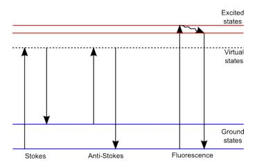
Figure 2.3: Visualization of Raman scattering and Fluorescence. Raman scattering leads to a constant frequency shift to higher (Anti-Stokes) or lower (Stokes) frequencies with respect to the pump light (independent of the pump frequency), while fluorescence results in the emission of photons at fixed frequencies.
