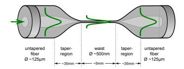
Figure 1.1: Sketch of a tapered optical fiber. Shown is the normal fiber (left and right) with the nanofiber in-between. The intensity distribution of light propagating in the fiber is shown in green. In the taper region, the light transitions from propagating in the core (light gray) to propagating in the cladding (dark gray) and the evanescent field is now in the surrounding vacuum. Note that the relative sizes of core, cladding and nanofiber are not to scale. Figure taken from [13].
