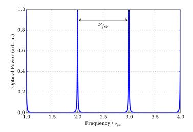
Figure 2.2: Longitudinal modes of an FPI with normalized power and a finesse of 100.
