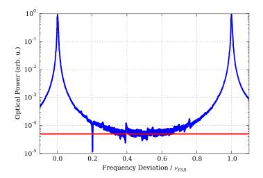
Figure 2.20: Transmitted intensity while scanning over one FSR. The peaks of the fundamental mode are at 0 and 1 and in-between no significant coupling to any transverse modes can be seen. This measurement is taken by coupling the light that exits the cavity into a single-mode fiber and measuring after the fiber. The red horizontal line indicates the calculated maximal suppression of  $-43.04\,\mathrm{dB}$ .
