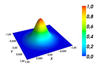
Figure 2.9: Shown is a two-dimensional Gaussian that describes the intensity distribution of a Gaussian beam. The normalized intensity is shown on the z-axis, while the x- and y-axes define a plane perpendicular to the direction of propagation. The beam's center is at position (x = 0, y = 0).
