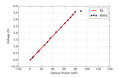
Figure 2.24: Power-Voltage characteristics of the photodiode. Saturation occurs at around  $80 \,\mu\text{W}$ . The slope of the fit is  $(4.52 \pm 0.02) \times 10^{-2} \,\mu\text{W} \,\text{V}^{-1}$
