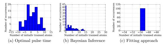
Figure 3.11: Results of using all three methods on datasets that contain only background counts but no signal counts.
