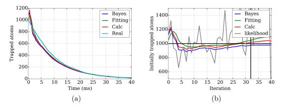
Figure 3.10: (a) Real-time estimation of the current number of trapped atoms along the nanofiber using a simulated measurement.
