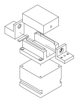
Figure 2.7: Exploded view of the cavity mount. The mirrors are placed in the holes of the two mounts in the slide rail. A plastic cap covers the setup to minimize disturbances and to protect the mirrors from dust. The mirror mount to the right is placed on a translation stage (not shown).
