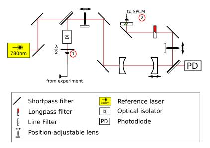
Figure 2.23: Experimental Setup of the Cavity Filter. The reference laser is shown in yellow and includes the saturation spectroscopy setup for its stabilization (cf. section 2.6.2). "PD" signifies a photodiode and "SPCM" a single-photon counting module. The arrows next to the lenses and the second cavity mirror indicate their mounting on translation stages.
