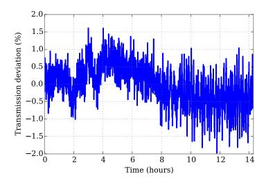
Figure 2.30: Long-term stability of the cavity transmission. Shown is the deviation from the mean value in percent.
