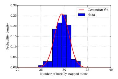
Figure 3.5: Fitting to the datasets of simulations with 30 atoms, whilst cooling them so that no atoms are lost. The measurement time is 200 ms and the mean value is 29.5 atoms with a standard deviation of 1.5 atoms.
