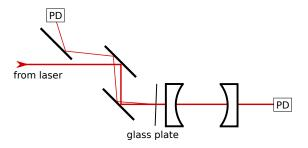
Figure 2.31: Schematic setup for transmission measurement. A glass plate is placed in front of the cavity at almost a right angle to least influence the coupling to the cavity. The reflection of the glass plate is then routed to a photodiode to measure the intensity changes before the cavity. Note that not the real intensity but only its relative changes are of interest for this measurement. The intensity after the cavity is measured with another photodiode.
