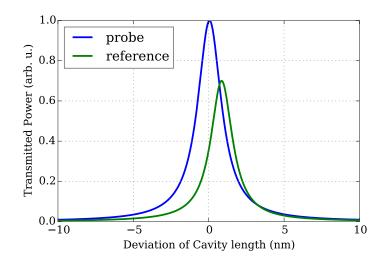
Figure 2.29: Ideal FSR for alignment of probe and reference laser transmission peaks. Shown are the transmitted powers of the probe and reference laser with changing distance between both mirrors of the cavity. The x-axis corresponds to the positional change of the second cavity mirror from a point at which the probe transmission is maximized.
