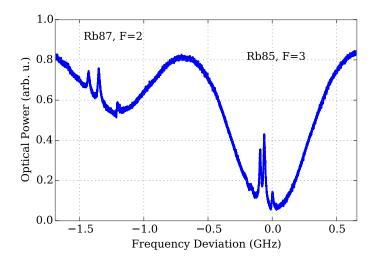
Figure 2.25: Saturation spectroscopy using a gas cell with Rubidium 87 and Rubidium 85. The x-axis shows the frequency deviation from the Rubidium 85 D2  $F = 3 \rightarrow F' = 4$  transition. The labels F = 2 and F = 3 refer to the ground state of the transitions.
