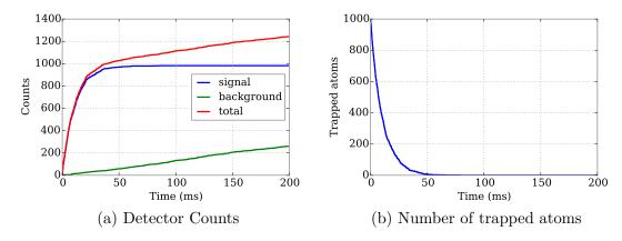
Figure 3.2: (a) Shown are the cumulative sums of the arrays for simulated signal counts and background counts. The background (green) shows a linear increase which is due to a constant rate of background counts (see text). The signal counts saturate when all atoms are lost.
