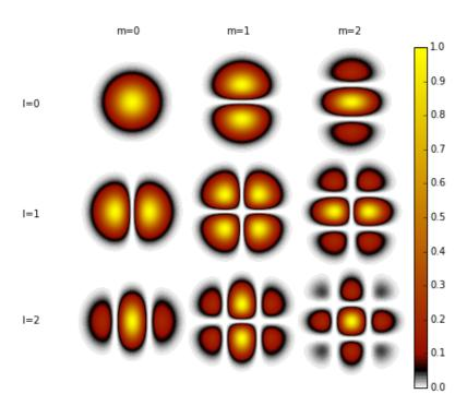
Figure 2.11: Visualization of Hermite-Gaussian modes of a resonator. Shown are the normalized color-coded intensity cross-sections of the beam.
