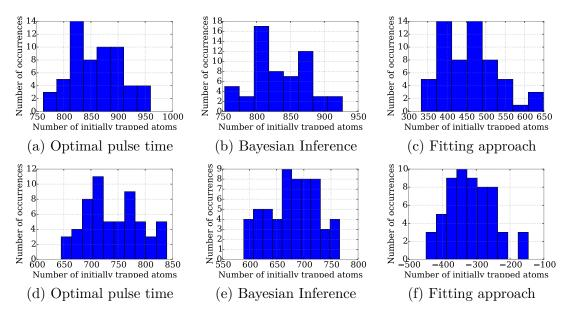
Figure 3.12: Results of using all three methods on datasets with 1000 atoms that contain very high background counts.
