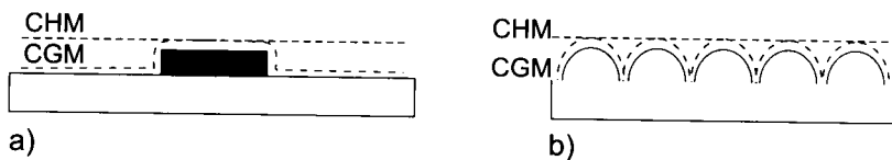
Fig. 15. – Schematic representation of the constant height mode (CHM) and constant gap mode (CGM) for tip-sample scanning. While CHM offers advantages for the sample in a) it creates complications for the one in b).
