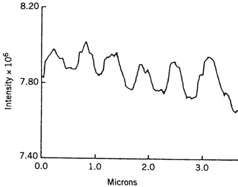
Figure 75: Intensity cross section of a line grating. [from Paesler/Moyer "Near-Field Optics"]
