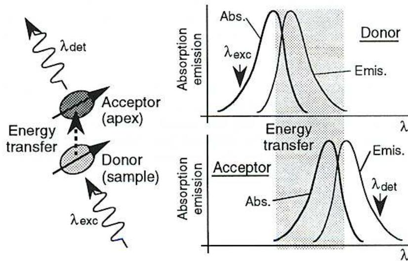
Figure 117: Schematics of Foerster Resonant Energy Transfer (FRET). [from Ohtsu, "Near-field Nano/Atom Optics and Technology"]
