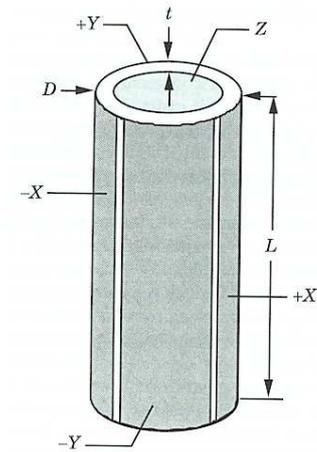
Figure 95: A four-segmented piezo tube. A SNOM tip is glued inside the tube. [from Paesler, Moyer "Near-Field-Optics"]
