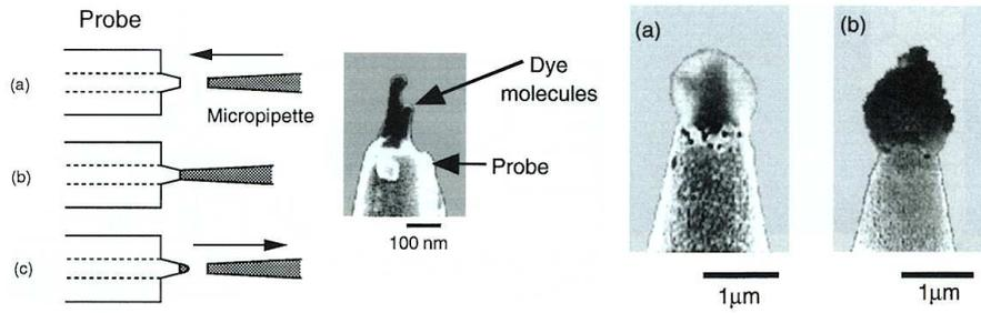
Figure 118: Fabrication of a functionalized SNOM probe (left), SEM-image of tips functionalized with PDA-Polymer (a) and GaAs powder (b). [from Ohtsu, "Near-field Nano/Atom Optics and Technology"]
