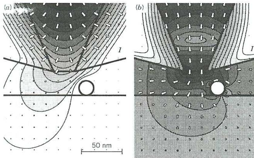
Figure 79: Calculated intensity in the near-field of an aperture above a perfectly conducting cylinder (multiple-multipole-method). [from Paesler, Moyer "Near-Field Optics"]
