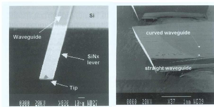
Figure 116: SEM image of one (left) and several (right) SiN SNOM cantilevers. [from P. Gall-Borrut et al., J. Mic. 202, 72 (2000)]
