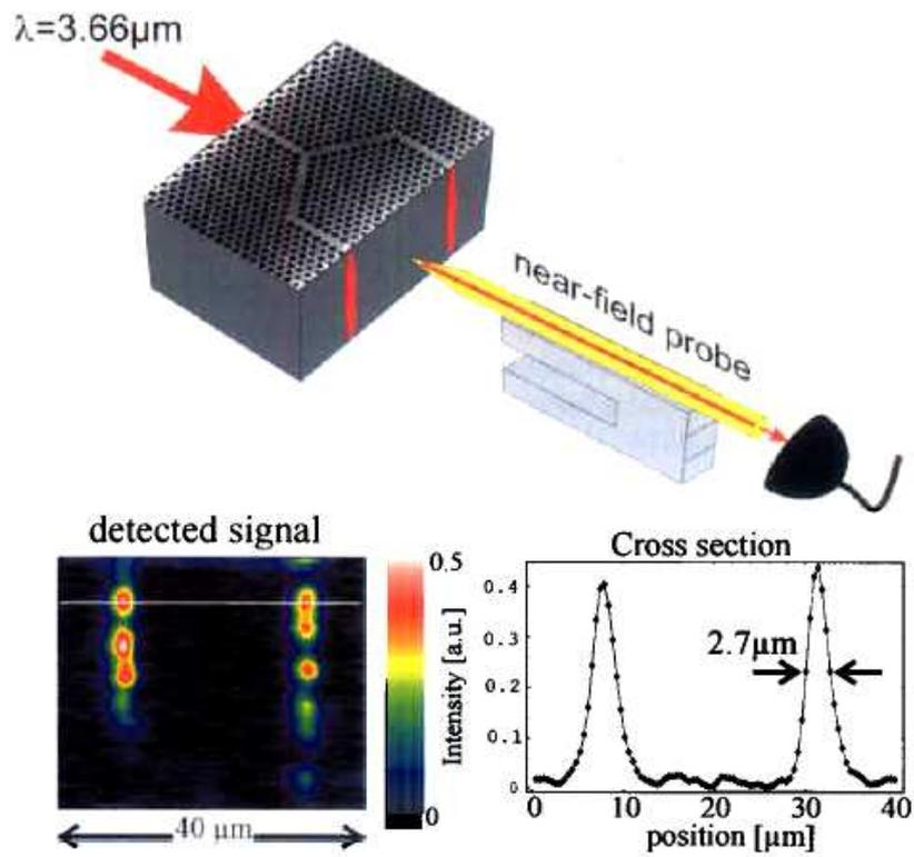
Figure 124: Investigation of the optical performance of a photonic crystal structure with a SNOM probe. [from V. Sandoghdar, "Trends and Developments in Scanning Near-field Microscopy"]
