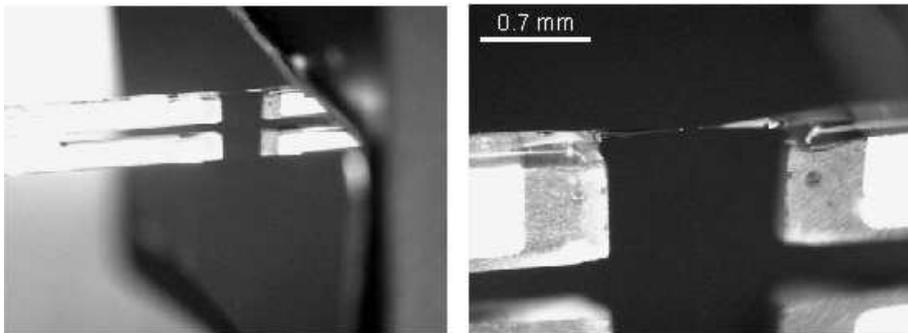
Figure 96: SNOM tip on a tuning fork.
