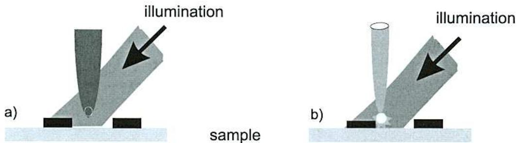
Figure 109: Schematics of apertureless SNOM: A scattering probe scatters near-fields locally at an object. [from V. Sandoghdar, "Trends and Developments in Scanning Near-field Microscopy"]
