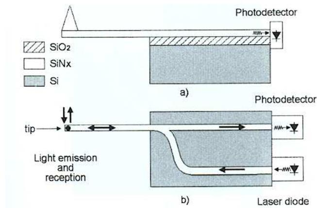
Figure 115: Design of an integrated structure consisting of a SNOM tip and a SiN-waveguide [from P. Gall-Borrut et al., J. Mic. 202, 72 (2000)]
