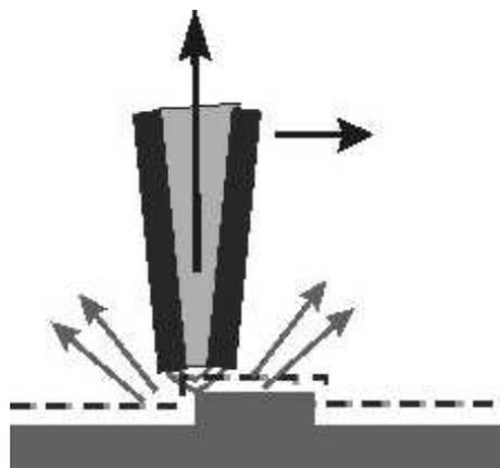
Figure 73: Principle of a modern realization of a SNOM aperture with the help of a metal coated optical fiber.
