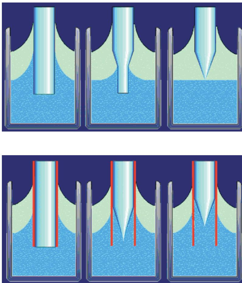
Figure 100: Turner etching (top) and tube-Etching (bottom).
