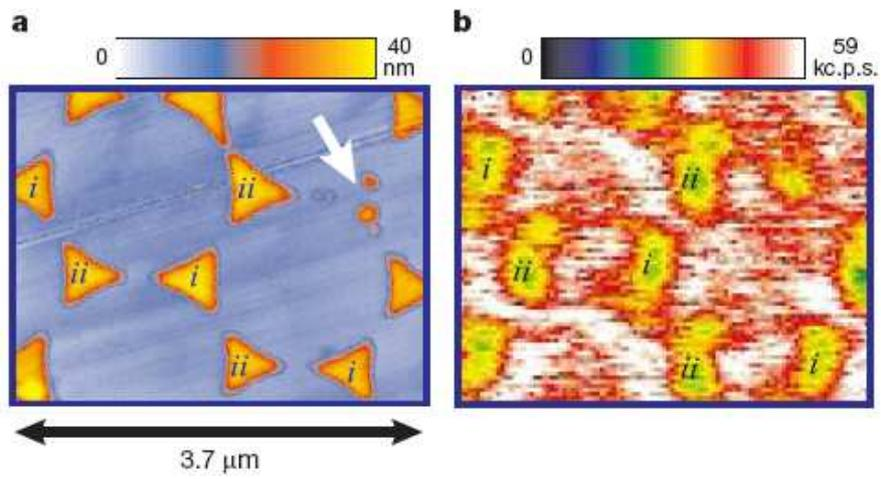
Figure 114: a) An atomic force microscope (AFM) topography image of the area of the sample; b) The optical raster-image recorded using the fluorescence of a single terrylene molecule for illumination. [from Hettich et al., Nature 405, 325 (2000)]
