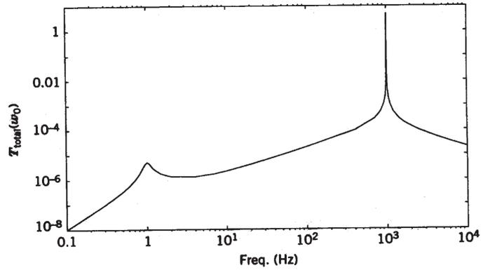
Figure 93: Resonance curve of a SNOM probe on an optical table. 1 Hz corresponds to the resonance of the table, 1 kHz to the resonance of the SNOM tip. [from Paesler, Moyer "Near-Field-Optics"]
