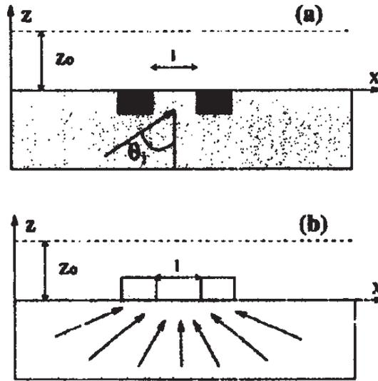
Figure 85: Numerical simulation: (a) two gold particle with  $w=\lambda/10$ ,  $h = \lambda/40$  in glass with  $l = \lambda/8$ ; (b) glass substrate with  $w=\lambda/4$ ,  $h = \lambda/40$  und  $l = \lambda/10$  [from Greffet, Carminati, Prog. Surf. Sci. 56, 133 (1997)]
