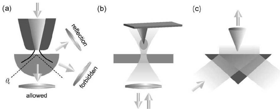
Figure 76: (a) aperture SNOM, (b) aperture-less SNOM, and (c) scanning tunneling microscopy. [from Hecht et al., J. Chem. Phys., 112, pp. 7761-7774 (2000)]
