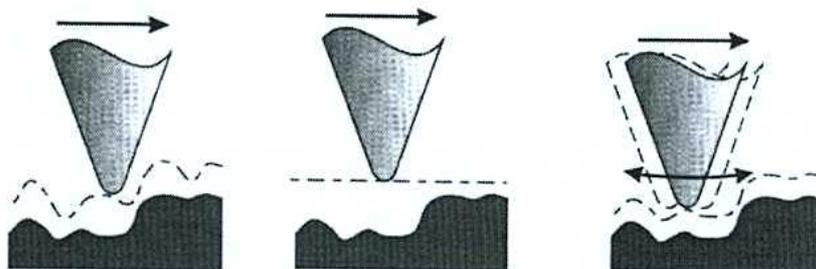
Figure 83: Constant intensity (left), constant height (middle) and constant distance (right) modus in SNOM [from Courjon, Bainier, Rep. Prog. Phys. 57, 989 (1994)]
