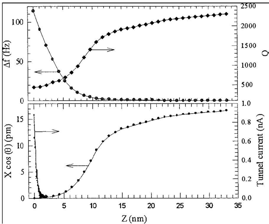
Figure 94: Change of resonance frequency, quality factor, and tunnel current of a metal coated tip during approach [Grober et al., Rev. Sci. Instr. 71, 2776 (2000)]
