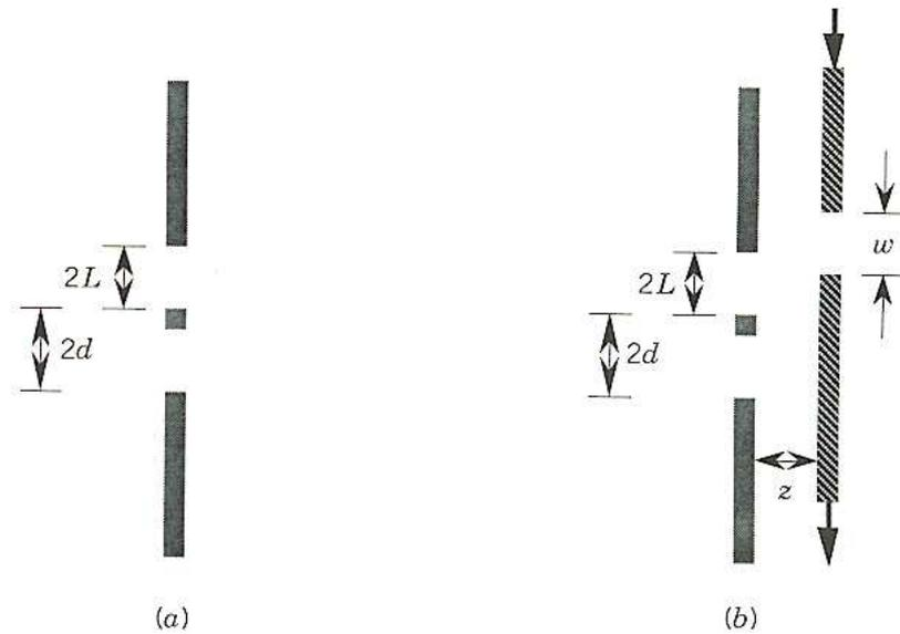
Figure 107: Model to study optical resolution with far-field (a) and near-field (b) microscopy. [from Paesler/Moyer, "Near-Field Optics"]
