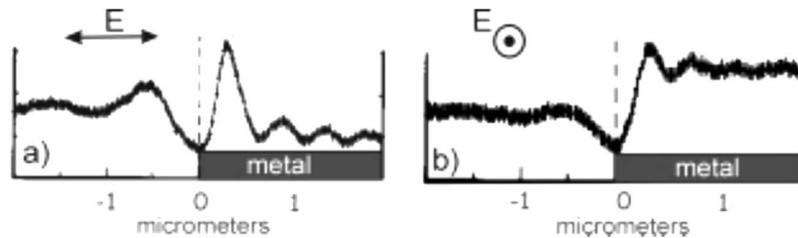
Figure 81: Measured signal of SNOM probe scanned across a metallic step for two different polarizations [from Huser, J. Opt. Soc. Am. A 16, 141 (1999)]
