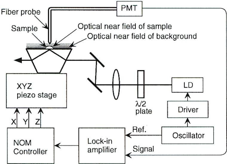
Figure 103: SNOM in Collection Mode [from Ohtsu, "Near-Field Nano/Atom Optics"]
