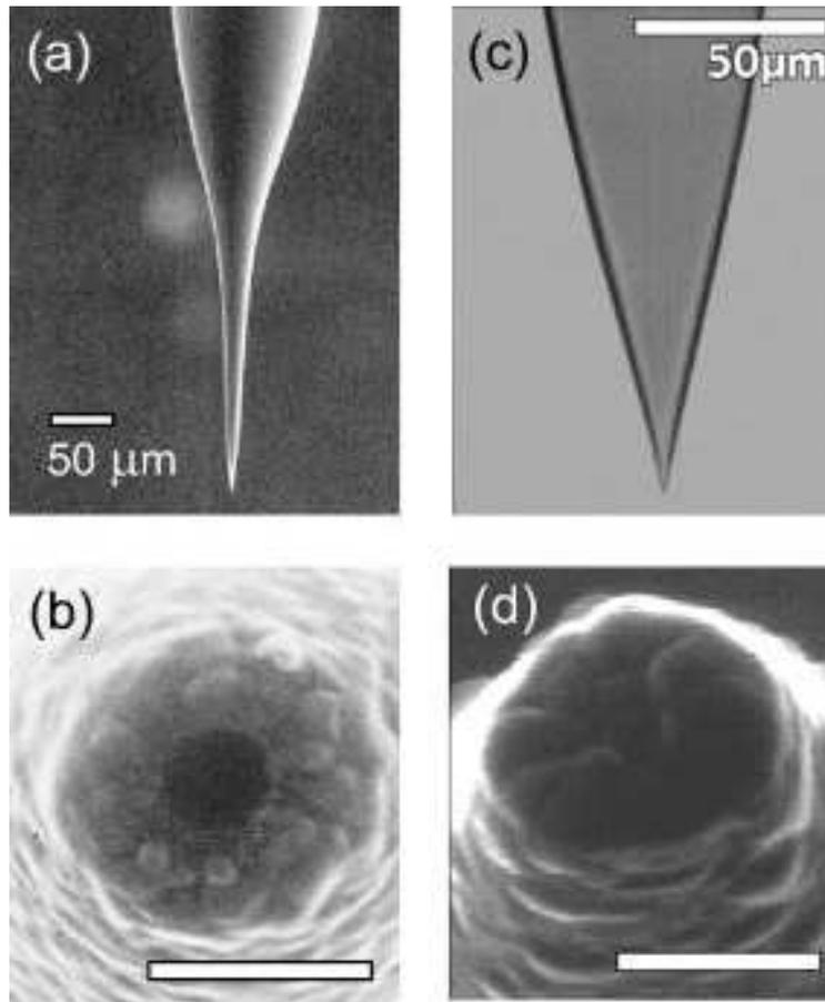
Figure 99: Optical (b) and SEM (a, c, d) pictures of pulled (left column) and etched (right column) SNOM tips. Scale bar = 300 nm. [from Hecht et al., *J. Chem. Phys.*, 112, pp. 7761-7774 (2000)]
