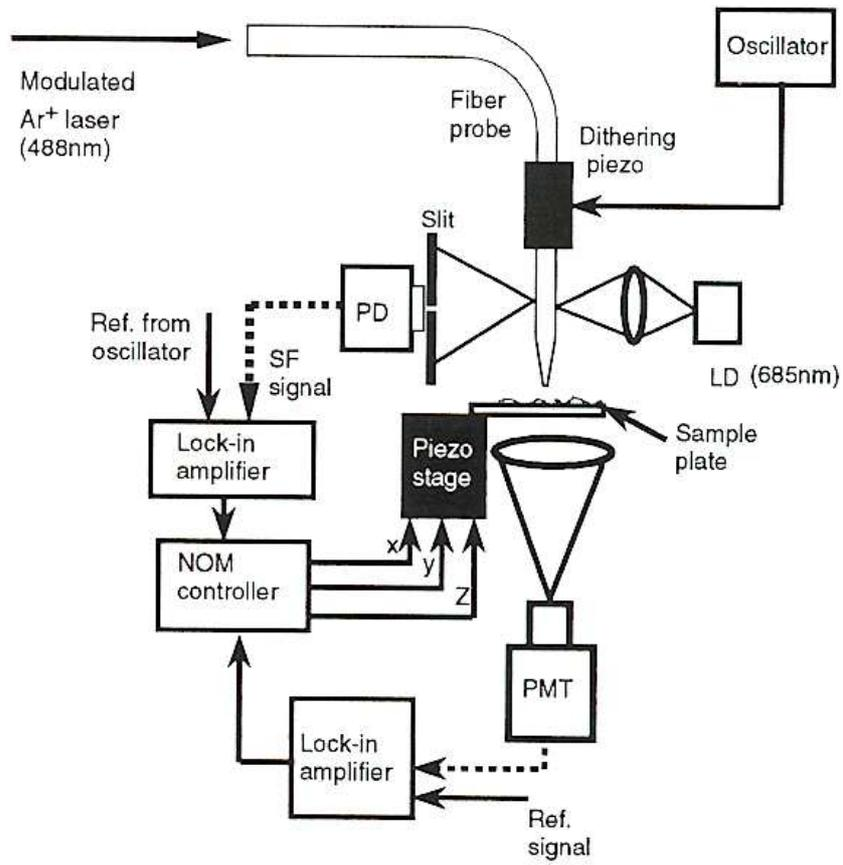
Figure 104: SNOM in Illumination Mode [from Ohtsu, "Near-Field Nano/Atom Optics"]
