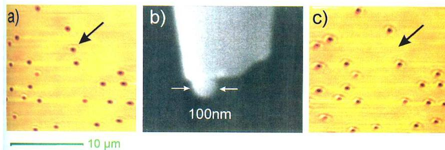
Figure 112: Attaching a gold particle to a SNOM tip. Middle: SEM image, Left and Right: microscope image. [from T. Kalkbrenner et al., J. Mic. 202, 72 (2000)]
