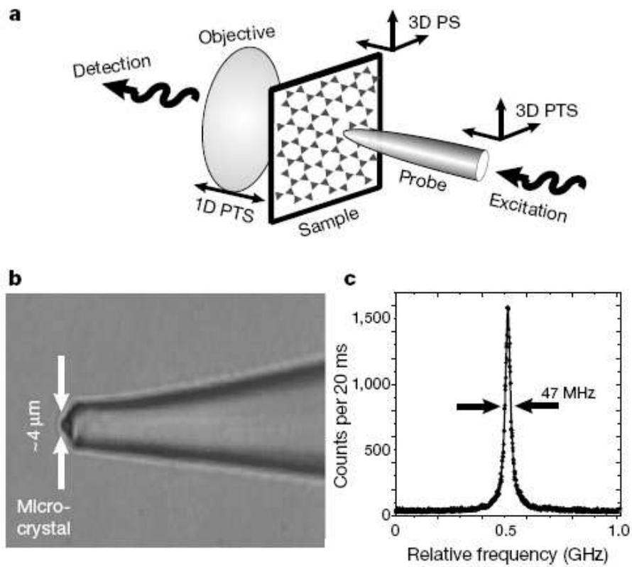
Figure 113: A single molecule as nanoscopic light source. a) Schematic view of the experimental configuration; b) an optical microscope image of the fibre probe displaying a micro-crystal of p-terphenyl glued to its end. The micro-crystal was lightly doped with terrylene molecules; c) An excitation spectrum of the molecule used for recording the images. [from Hettich et al., Nature 405, 325 (2000)]
