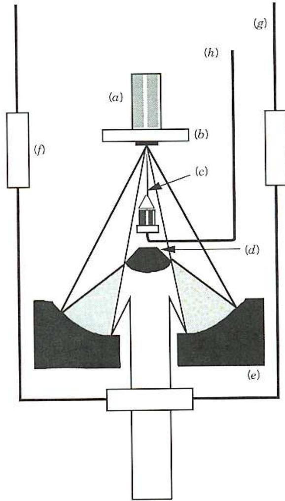
Figure 105: Low-temperature SNOM in a cryostat; (a): Piezo-tube scanner, (b):Sample, (c): SNOM tip, (d): illumination mirror, (e): parabolic mirror, (f): window, (g): cryostat, (h): optical fiber [from Paesler, Moyer "Near-Field-Optics"]
