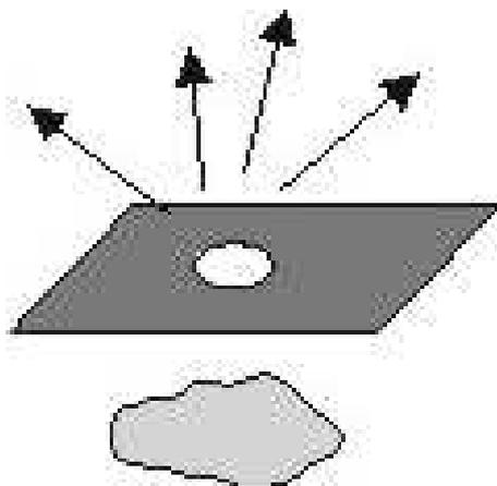
Figure 72: Cartoon picture of Synge's idea: A tiny aperture is scanned across an object and detects the optical near-field. A resolution below the Rayleigh limit is obtained in this way.
