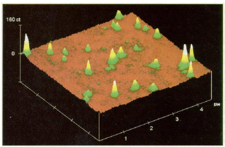
Figure 120: SNOM image of single Oxazin 720 molecules. The optical resolution in this image is approx. 100 nm.
