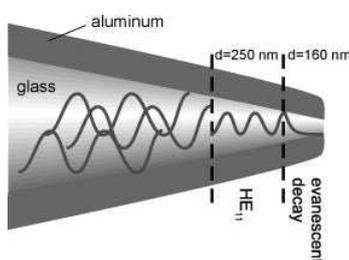
Figure 98: Schematics of light transmission through an aperture probe [from Hecht et al., J. Chem. Phys., 112, pp. 7761-7774 (2000)]
