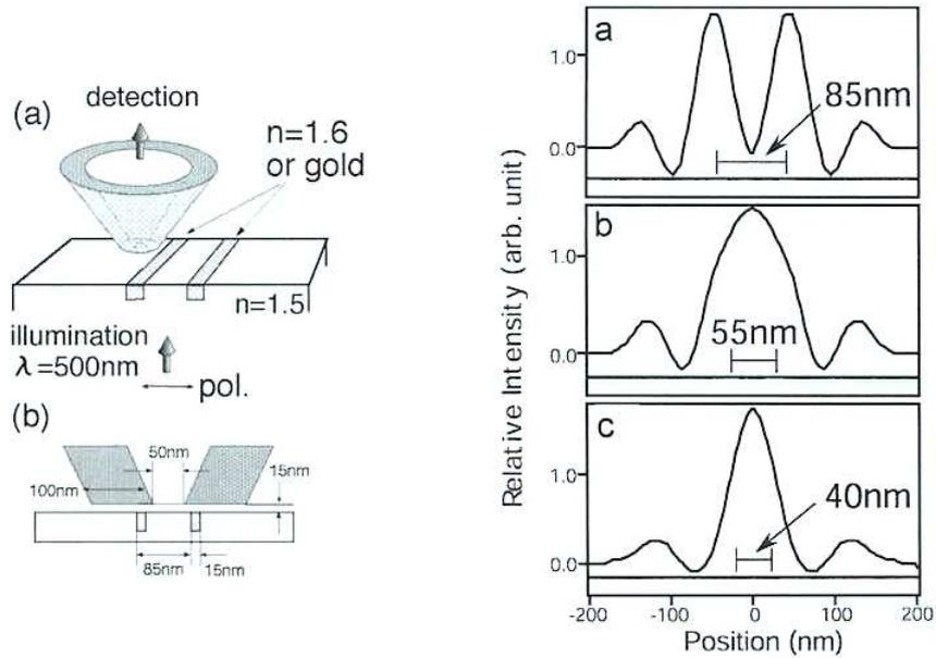
Figure 80: Signal when scanning across two dielectric stripes (calculated by the FDTD method). [from Kawata, Ohtsu, Irie "Nano-Optics"]
