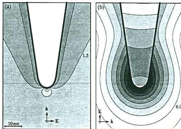
Figure 110: Local field enhancement at a gold tip (curvature radius 5 nm) for two different polarizations of the illumination.
