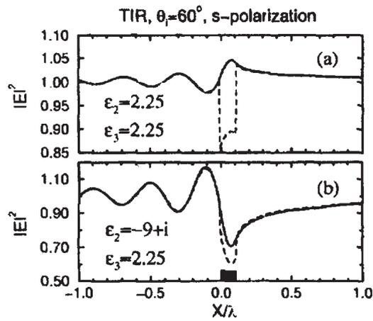
Figure 89: Same as above, but with illumination under an incidence angle of  $60^\circ$ . Solid: Constant height mode with  $d = 0.0225\lambda$ ; Dashed: Constant distance mode with  $d = 0.0075\lambda$ . [from Greffet, Carminati, Prog. Surf. Sci. 56, 133 (1997)]
