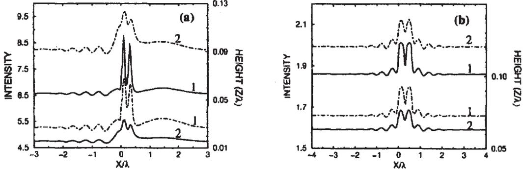
Figure 86: (a) Corresponding to fig. 85 (a). Constant intensity curves (dashed) and constant height curves (solid) for two different distances  $z_0 = 0.03\lambda$  (curves 1) and  $z_0 = 0.09\lambda$  (curves 2); (b) Corresponding to fig. 85 (b) with  $z_0 = 0.07\lambda$  (curves 1) and  $z_0 = 0.12\lambda$  (curves 2). [from Greffet, Carminati, Prog. Surf. Sci. 56, 133 (1997)]
