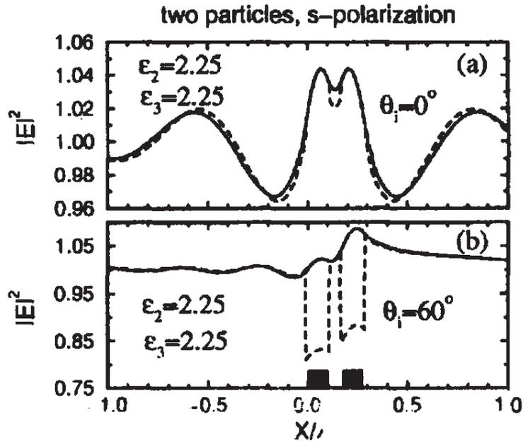
Figure 90: Calculated near-field signal above two bars of width  $w = 0.1\lambda$ , height  $h = 0.015\lambda$  and distance  $l = 0.075\lambda$  for two different  $\varepsilon$  at  $0^\circ$  and  $60^\circ$  angle of incidence of illumination. Solid: Constant height mode with  $d = 0.0225\lambda$ ; Dashed: Constant distance mode with  $d = 0.0075\lambda$ . [from Greffet, Carminati, Prog. Surf. Sci. 56, 133 (1997)]
