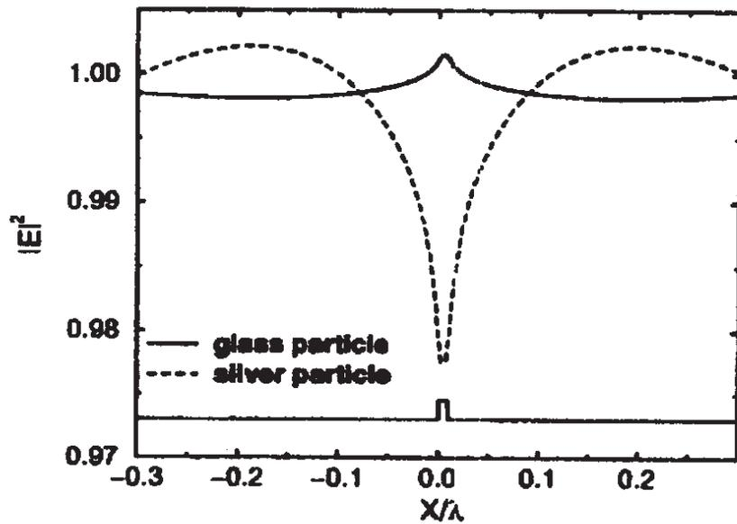
Figure 77: Calculated intensity  $4 \text{ nm}$  above a  $2 \times 6 \text{ nm}$  silver wire (dashed) and a glass wire (solid) [from Greffet, Carminati, Progr. Surf. Sci., 56, 133 (1997)]
