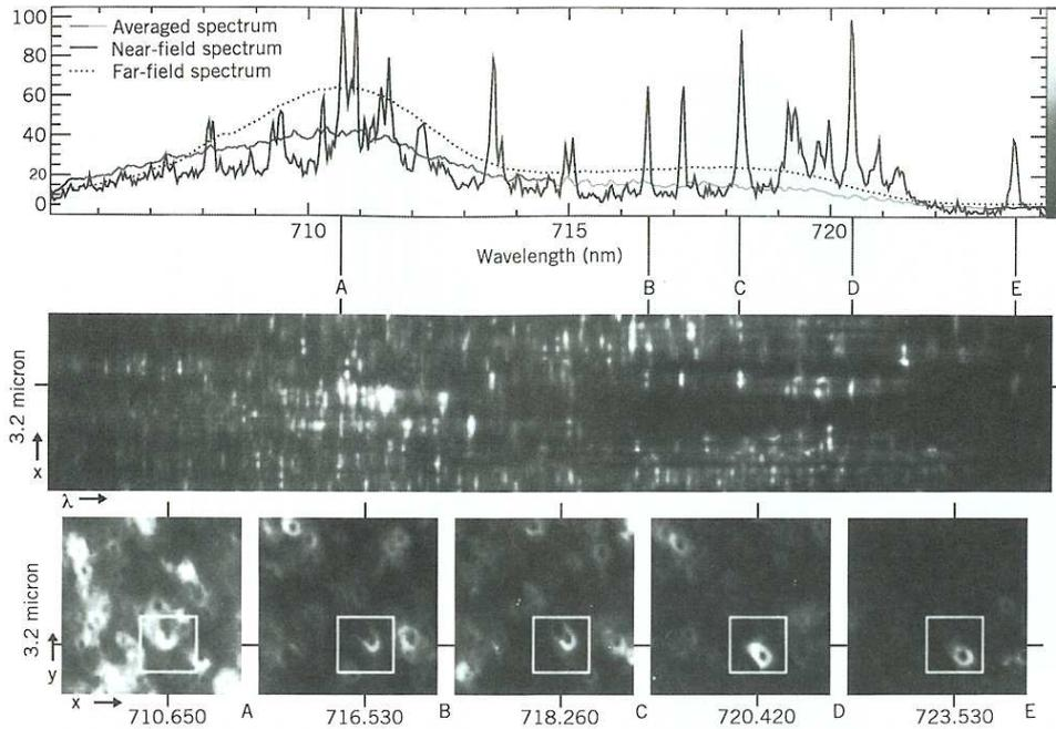
Figure 122: Investigation of localized excitation in a semiconductor quantum film, so-called natural quantum dots with SNOM. a) Near-field spectrum, b) near-field image, c) spectrally filtered near-field [from Hess et al., Science 264, 1740 (1994)]
