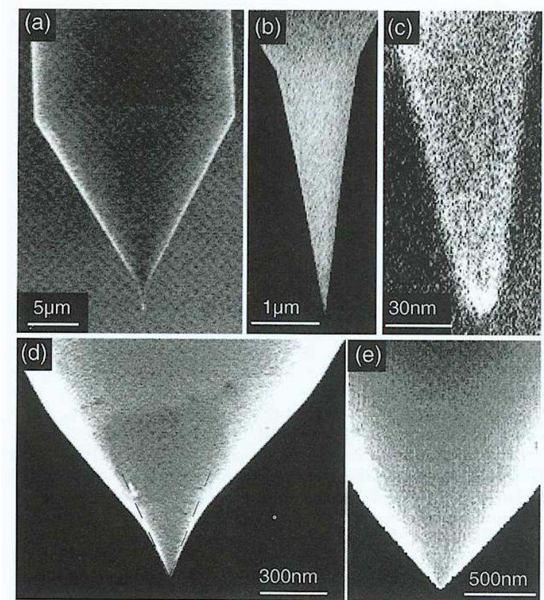
Figure 101: SEM-images of various etched fiber tips. [from Ohtsu, "Near-Field Nano/Atom Optics"]
