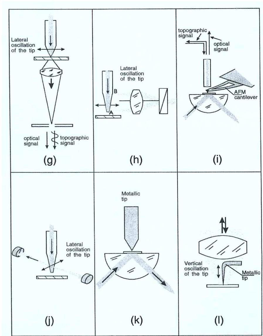
Figure 92: Different configurations in near-field microscopy. [from Courjon, Bainier, Rep. Prog. Phys. 57, 989 (1994)]
