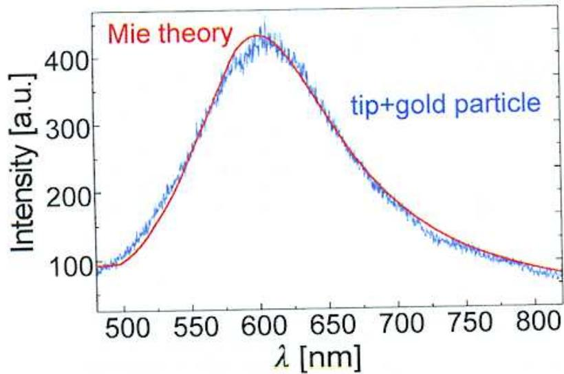
Figure 111: Measured and calculated plasmon resonance of a spherical gold particle at a SNOM tip. [from T. Kalkbrenner et al., J. Mic. 202, 72 (2000)]
