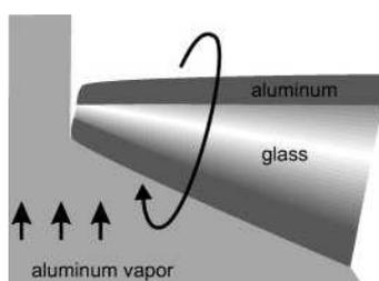
Figure 97: Schematics of metal-coating a SNOM tip [from Hecht et al., J. Chem. Phys., 112, pp. 7761-7774 (2000)]
