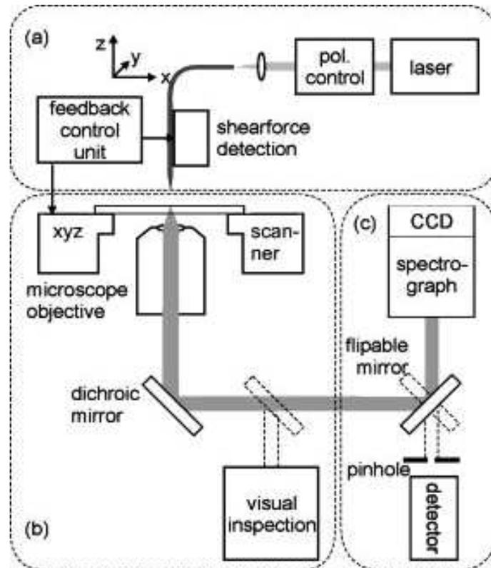
Figure 91: A typical SNMO setup in illumination/collection mode [from Hecht et al., J. Chem. Phys., 112, pp. 7761-7774 (2000)].
