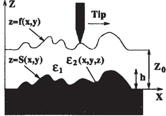
Figure 87: Geometry in constant distance mode. [from Greffet, Carminati, Prog. Surf. Sci. 56, 133 (1997)]
