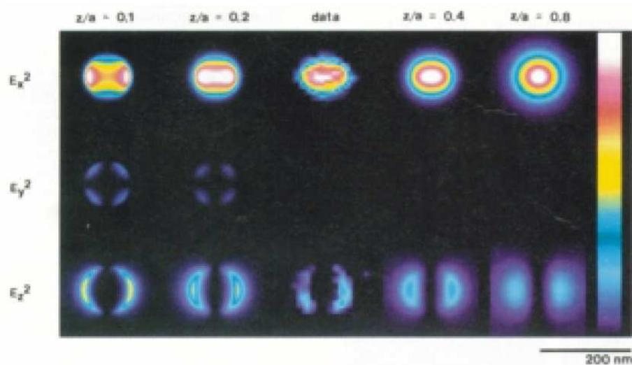
Figure 78: Calculated intensity of  $x$ -polarized light at a small aperture according to the Bethe-Bouwkamp-Theorie ( $a$ =diameter of aperture,  $z$ =distance from aperture) [from Betzig, Chichester, Science 262, 1422 (1993)]
