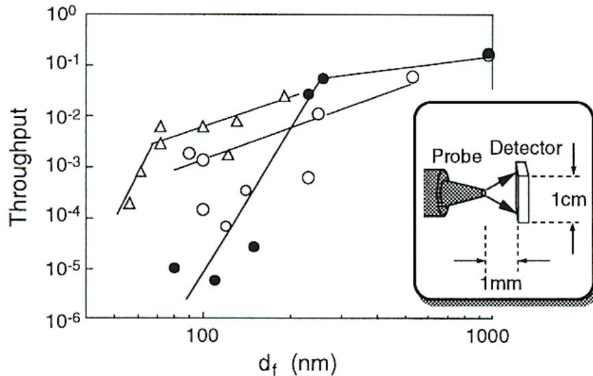
Figure 102: Measured transmission of different SNOM tips. Filled circles; conventional tips, open circles and triangles: high-throughput tips [from Ohtsu, "Near-Field Nano/Atom Optics"]
