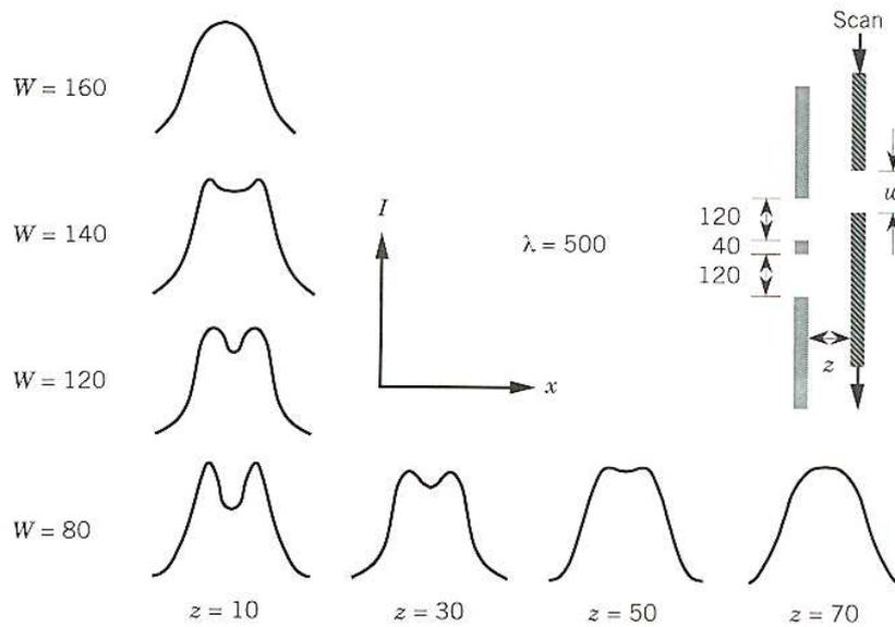
Figure 108: Calculated images of a double-slit in the near-field for different dimensions of the aperture and different distances  $z$  of the aperture from the slit. [from Paesler/Moyer, "Near-Field Optics"]
