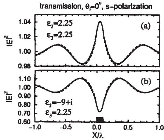
Figure 88: Calculated near-field signal above a bar of width  $w = 0.1\lambda$  and height  $h = 0.015\lambda$  for two different  $\epsilon$  and illumination under normal incidence. Solid: constant height mode with  $d = 0.0225\lambda$ ; Dashed: constant distance mode with  $d = 0.0075\lambda$ . [from Greffet, Carminati, Prog. Surf. Sci. 56, 133 (1997)]
