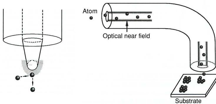
Figure 119: Proposal to trap single atoms in the optical field at the end of a near-field probe (left) or to "nano-deposit" clusters of atoms with hollow-core optical fibers. [from Ohtsu, "Near-field Nano/Atom Optics and Technology"]
