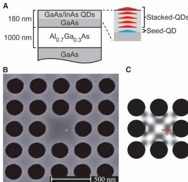
**Fig. 1.** (A) Schematic cross section of the semiconductor heterostructure. (B) SEM image of the S1-PC defect region in device I. The small white dot is the top QD of the targeted seed stack. (C) Plot of the electric field intensity present in the semiconductor of the S1-PC defect region, calculated by three-dimensional finite-difference time domain (25). Cavity-mode maxima correspond to darker gray levels. The red cross indicates the position of the seed stack.
