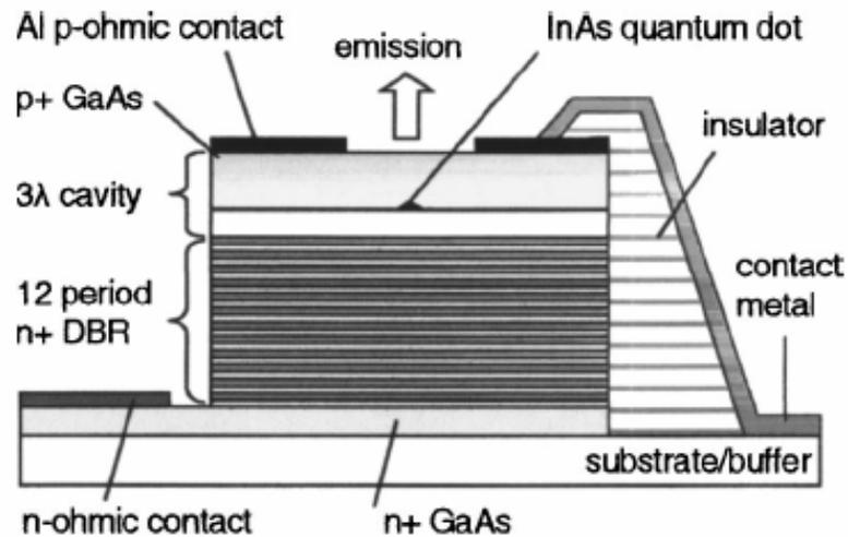
Left: Schematic of the device structure. A single QD within a cavity (formed by a Bragg mirror and the top interface) is isolated with an aperture in the metallic contact. The cavity enhances the collection efficiency of photons.
