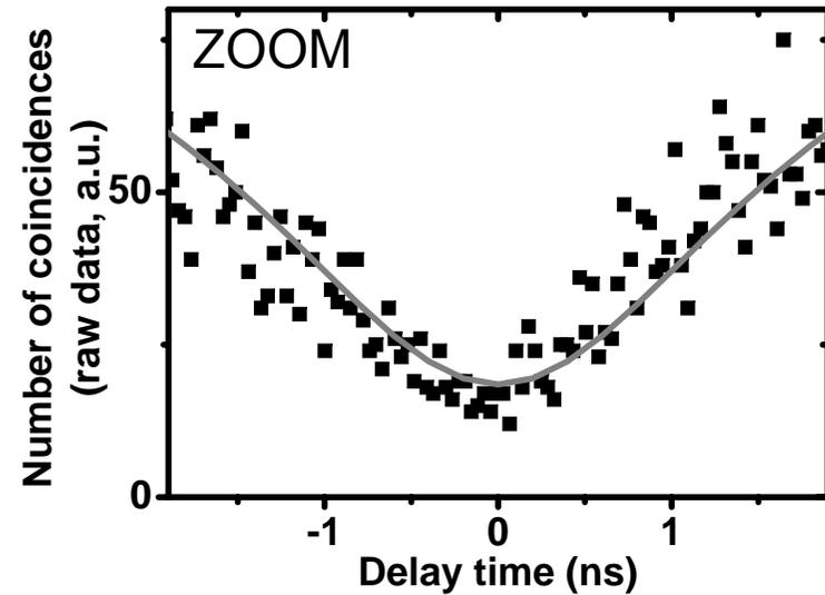
Measurement of  $g^{(2)}(\tau)$  under cw and pulsed optical excitation:
