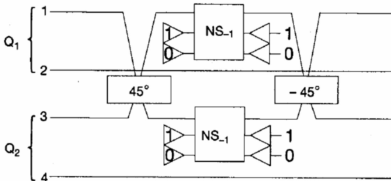
construction of a CZ gate with two  $NS_{-1}$  gates
