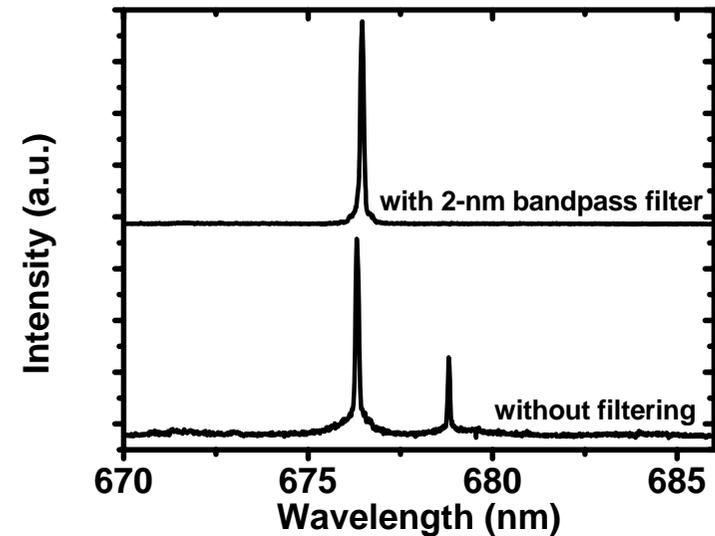
The additional mirror increases the photon emission rate by more than a factor of 2!.
