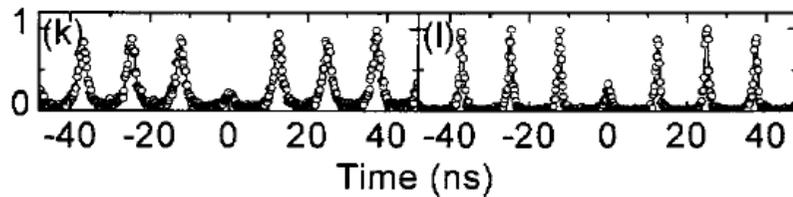
Under pulsed electrical excitation antibunching is observed both from the exciton (k) and from the biexciton (l). The lines are filtered out with a monochromator.
