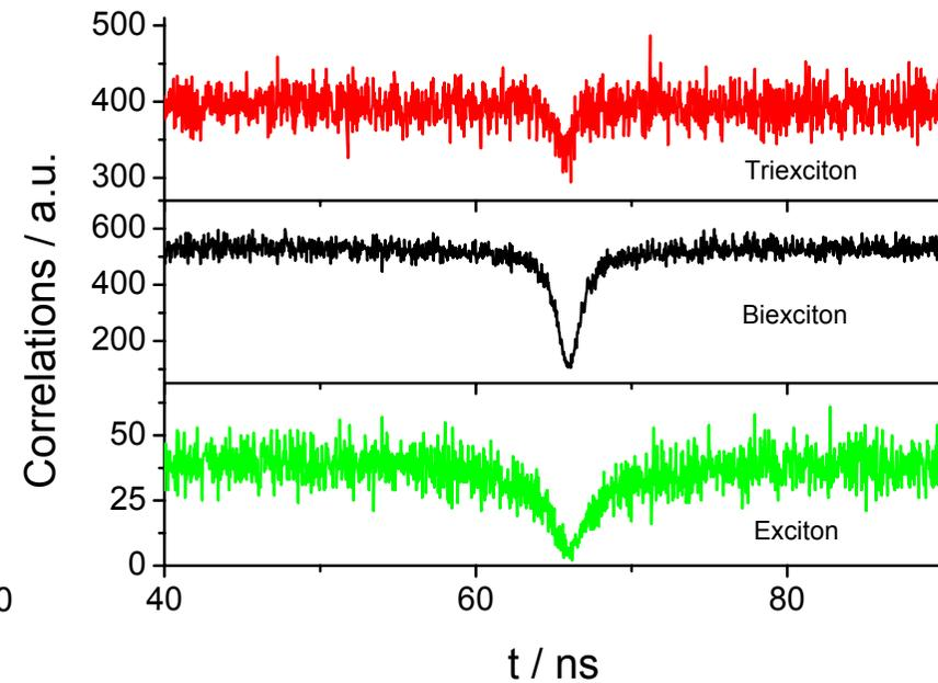
$g^{(2)}$  measurements for individual spectral lines
