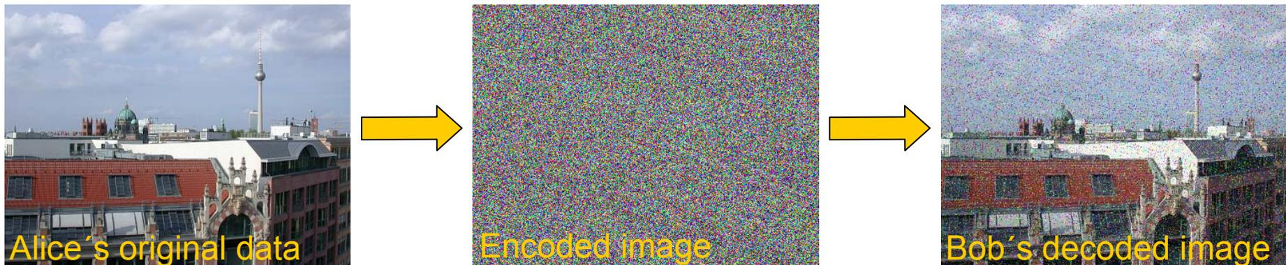
Transmission to Bob: 30 successful counts/s at a laser modulation of 20 kHz
