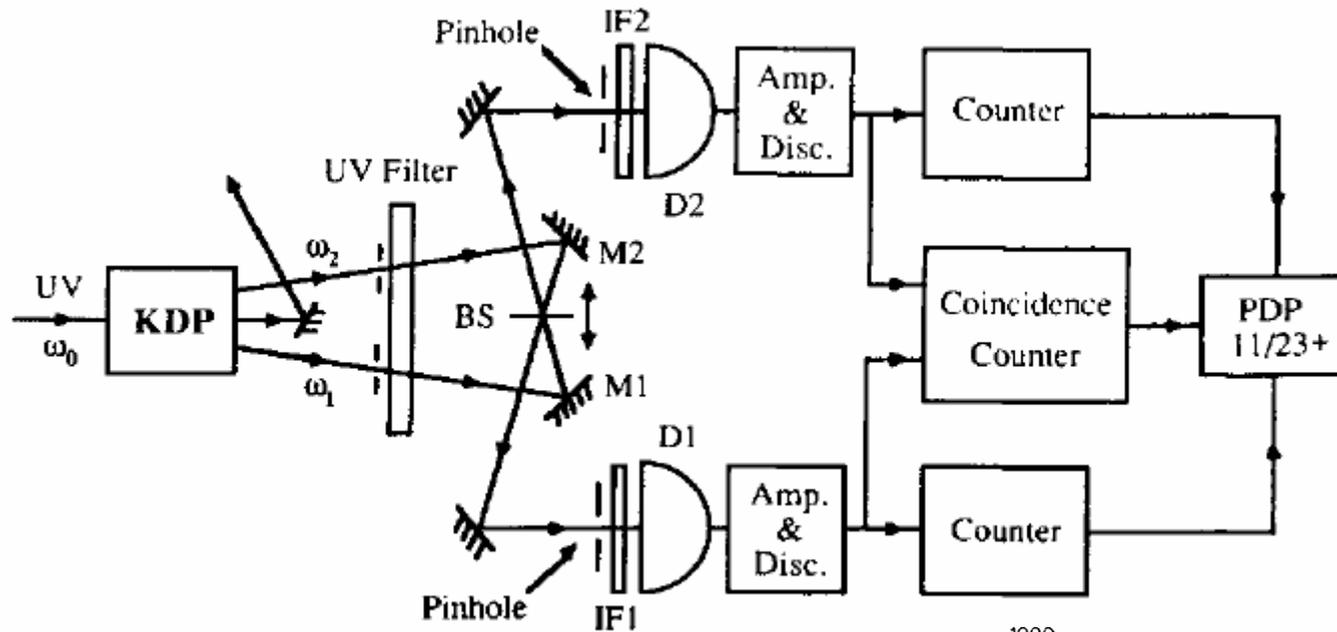
The depth of the HOM dip gives the „degree of indistinguishability“ of two photons.
