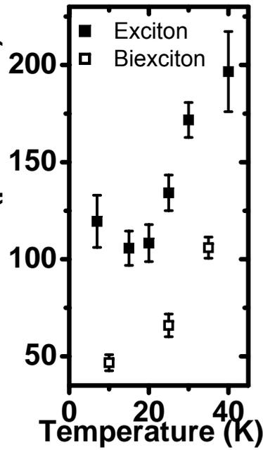
linewidth increases by a factor of two by increasing temperature from 7 to 40 K
