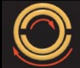
Circular currents flow in split-ring resonators (SRRs).
