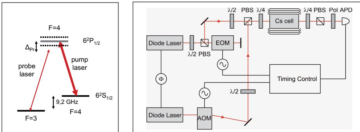
Figure 62: Left: Energy level diagram of  $^{133}\text{Cs}$ ; Right: schematic of an experimental setup.
