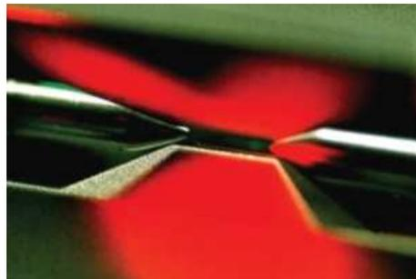
Figure 133: Close-up of a linear ion trap [from <http://heart-c704.uibk.ac.at/>].
