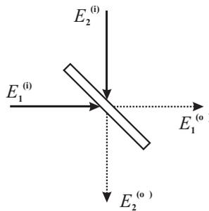
A classical beamsplitter can be described as a  $2 \times 2$  matrix that relates the input fields  $E_1^{(i)}$ ,  $E_2^{(i)}$  to the output fields  $E_1^{(o)}$ ,  $E_2^{(o)}$ .
