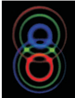
Figure 39: Photo of Photons from type-II down conversion in a BBO crystal [from http://www.quantum.univie.ac.at/ ]
