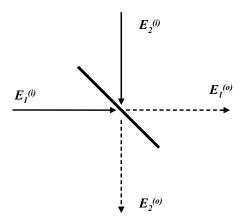
A classical beamsplitter can be described as a  $2 \times 2$  matrix that relates the input fields  $E_1^{(i)}$ ,  $E_2^{(i)}$  to the output fields  $E_1^{(o)}$ ,  $E_2^{(o)}$ .
