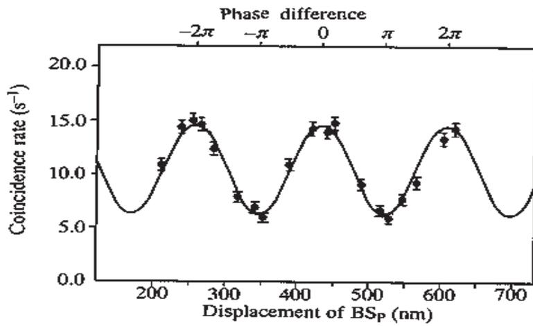
Figure 33: Experimental results of a two-photon interference experiment. Top: single photon rate; bottom: Two-photon coincidence rate [from Ou, et al., Phys. Rev. A 41, 566 (1990)]
