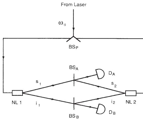
Figure 32: Setup of a two-photon interference experiment [Ou et al., Phys. Rev. A 40, 1428 (1989)]
