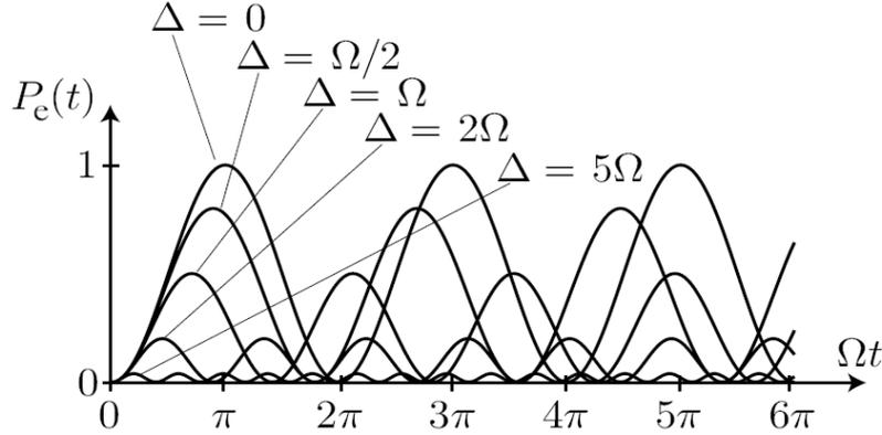
Figure 52: Time evolution of the probability  $P_e(t)$  to find the atom in the excited state for different detunings  $\Delta$ . [from D.A. Steck *Quantum and Atom Optics*]
