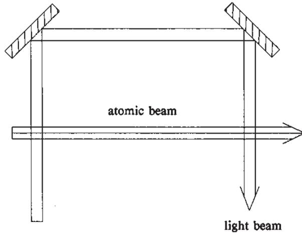
Figure 49: Principle setup for a Ramsey measurement.
