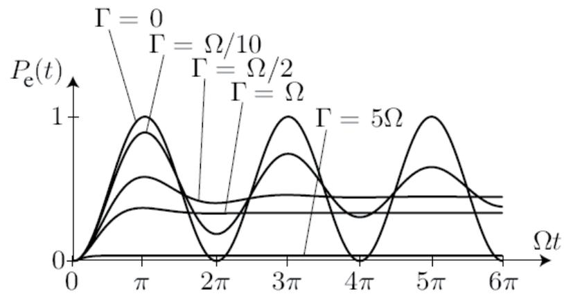
Figure 53: Time evolution of the probability  $\rho_{ee}(t)$  to find the atom in the excited state for different damping rates  $\Gamma$ . [from D.A. Steck *Quantum and Atom Optics*]
