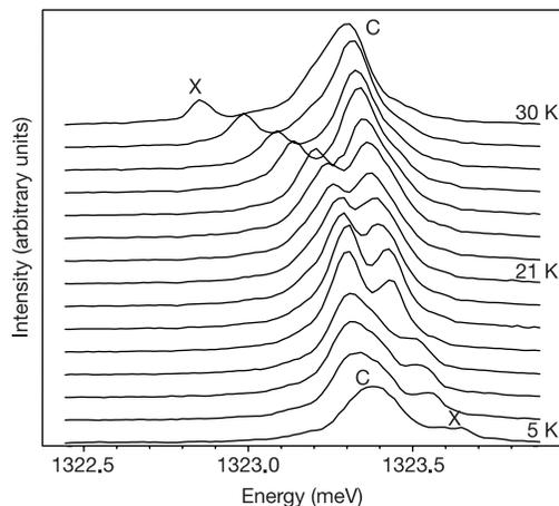
**Figure 3** Temperature dependence of photoluminescence spectra for a 1.5- $\mu\text{m}$  microcavity ( $Q = 7,350$ ) showing the tuning of a single QD exciton through resonance with the cavity mode. A clear anti-crossing is observed owing to strong coupling between the QD exciton and the microcavity photon mode.
