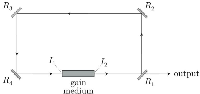
Since the cavity has a ring configuration, light passes through the gain medium in one direction only. Starting with the single-pass gain relation for a medium of length  $l_g$ ,
