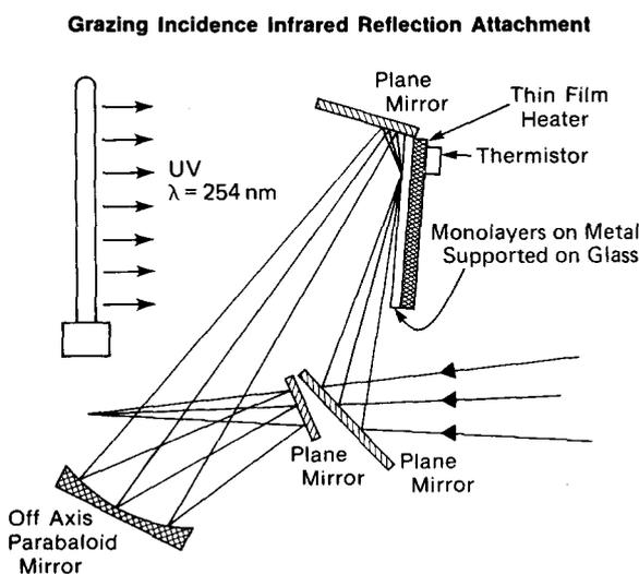
FIG. 1. Schematic of the grazing incidence reflection attachment with sample heater and UV lamp.
