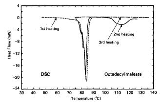
FIG. 2. Differential scanning calorimetry (DSC) thermogram for first and second heating of bulk Cd-octadecylmaleate (Cd-ODM), obtained at a heating rate of  $2 \,^{\circ}$ C min<sup>-1</sup>.
