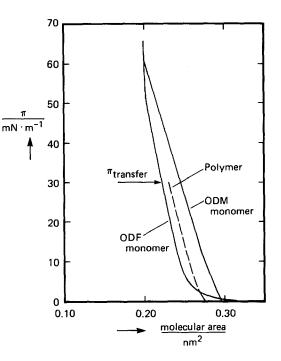
FIG. 3. Surface pressure vs area at room temperature for the monomers of Cd-octadecylfumarate (Cd-ODF) and Cd-octadecylmaleate (Cd-ODM) as well as for the common polymer.
