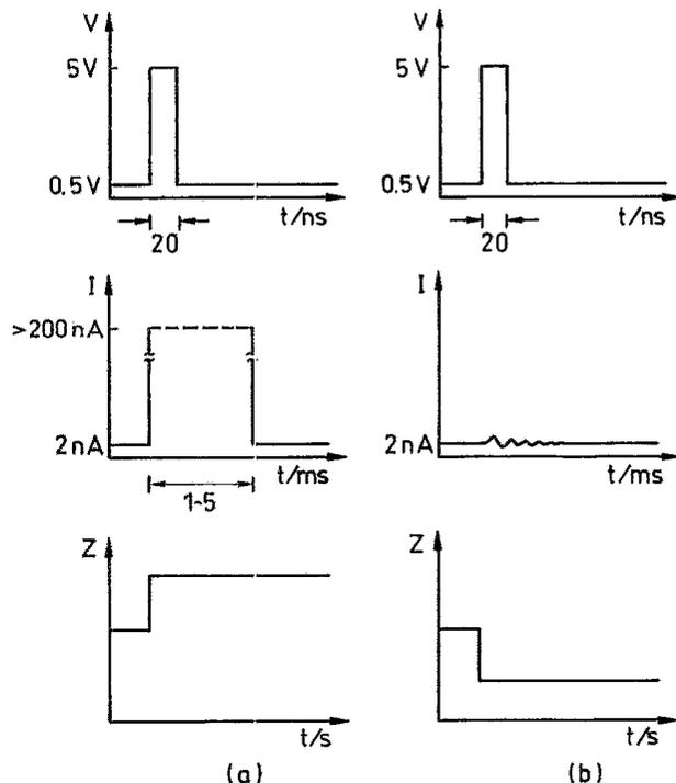
FIG. 4. Bias, current and z piezo position during surface modification by negative bias pulses applied with the STM. (a) without point contact formation and (b) with point contact formation.
