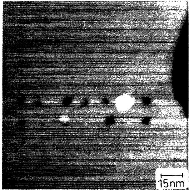
FIG. 2. STM images of Ag(111) on mica with eleven marks of about 10 nm diameter produced on two horizontal rows at positive sample bias. While generally a hole is formed, in two cases some material is transferred back to the surface, causing a hillock to be produced. Image size: 130 nm  $\times$  130 nm.
