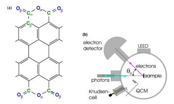
FIG. 1. (Color online) (a) Molecular structure of PTCDA (3,4,9,10-perylene tetracarboxylic dianhydride) with chemically inequivalent carbon and oxygen atoms. (b) Experimental setup at the x-ray standing-wave beamline ID32 (ESRF).
