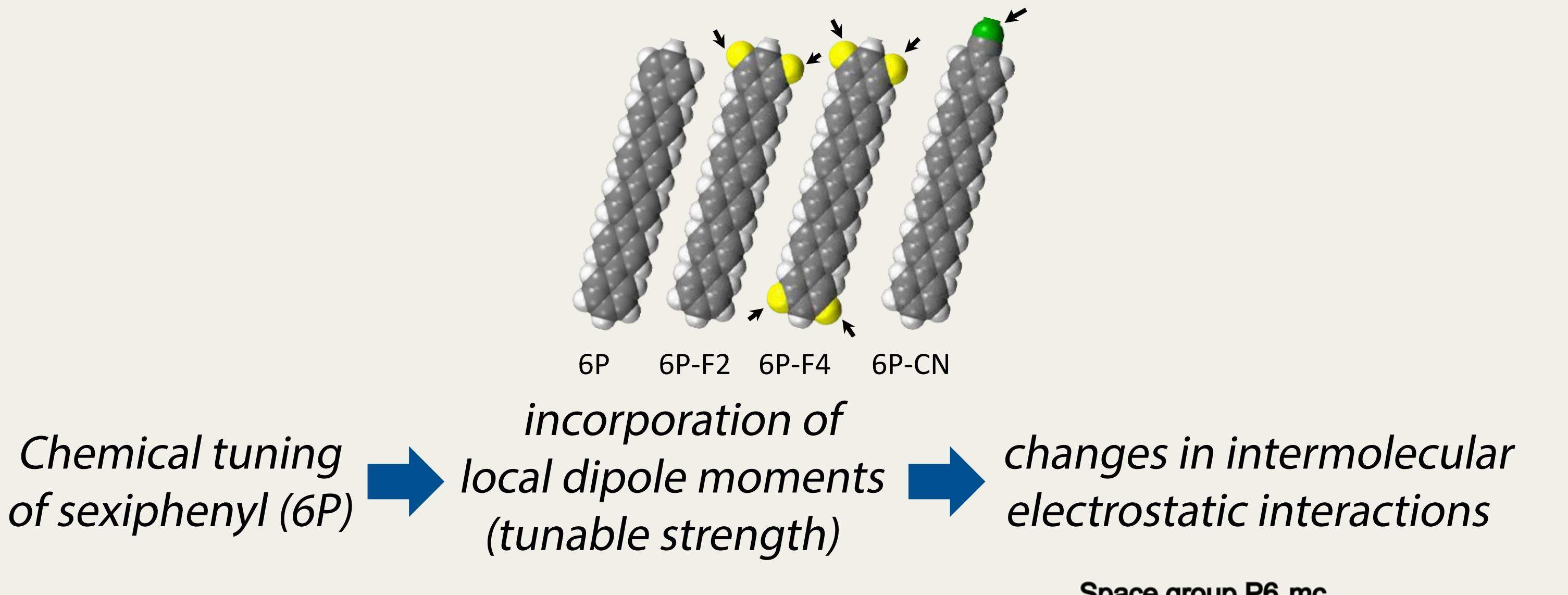
We study the growth of 6P and its derivatives on ZnO (1010) as a model HIOS system. The beneficial optical properties of 6P, e.g. fluorescence, are not affected by the chemical tuning. The deposition of the molecules was performed by OMBD in UHV ( $\sim 10^{-10}$  mbar) conditions.
