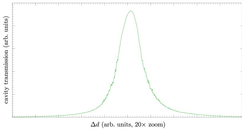
From these plots, find the FSR, finesse, resolution  $\delta\nu_{\text{FWHM}}$ , and  $Q$ -factor of the cavity.
