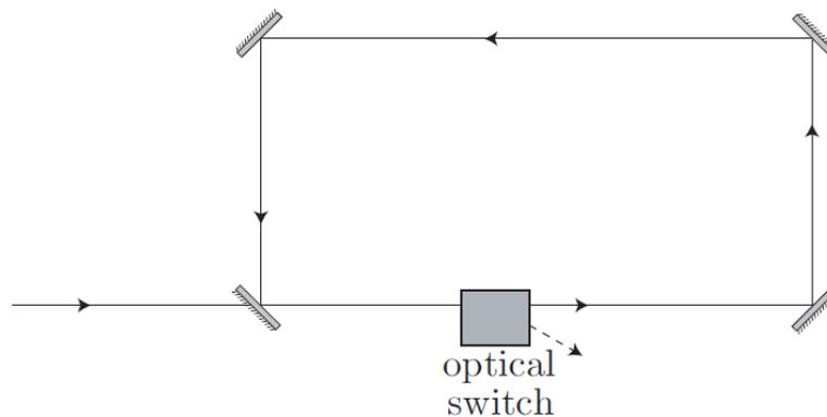
The cavity dumper operates as follows: the input light is turned on, and the circulating light builds up in the cavity to a large intensity. Then the optical switch is activated, deflecting the circulating intensity out of the cavity.
