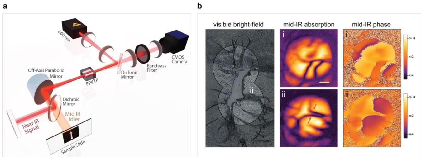
**a. Experimental Setup:** Wide-field imaging with undetected photons. **b. Bioimaging:** Imaging of a histology sample of a mouse heart with bright field microscopy, and absorption and phase imaging obtained with quantum microscopy with undetected photons.
