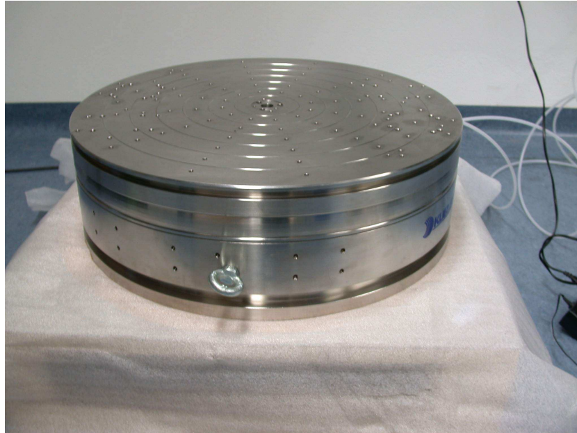
Figure 4.19: Precision turntable for rotating the laser stabilization setup for R1. Specifications are given in Table 4.5.
